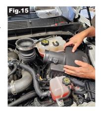
Step 13. Attach the coupler back to the air cleaner lid, ensuring a secure connection with the factory clamps. Reconnect the MAF sensor to its original position as shown in (Fig. 16).
