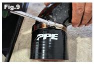
2: Loosely install the second clamp over the coupler. (Fig. 10)
