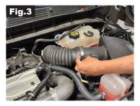
Step 5. Loosen the clamps securing the intake boot and remove the air cleaner lid and filter. (Fig. 4)
