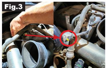
**Step 4.** Remove the CCV vent hose by following these steps:
