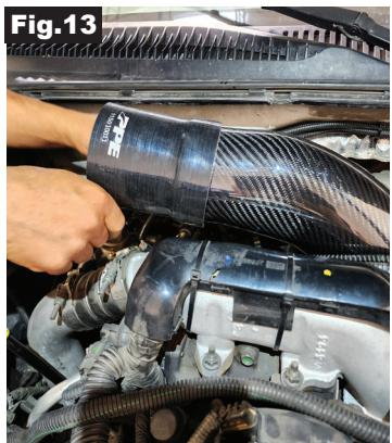
Step 14. Insert the trimmed air duct into the coupler and attach T-Bolt Clamps. **B** (Fig. 14)
