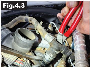
Step 5. Loosen the V-Band Clamp and remove the factory inlet duct from the turbo. (Fig. 5)
