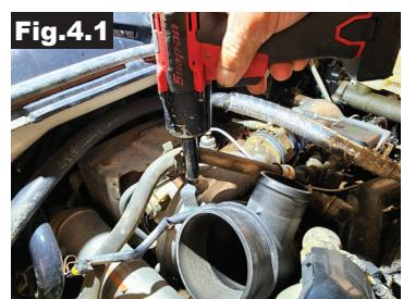
4.2. Remove the bolt securing the line to the PCV port. (Fig. 4.2)
