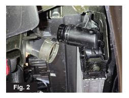
For both sides, disconnect factory intercooler hoses from factory intercooler pipes. Remove both factory intercooler hoses. (Fig. 3)
