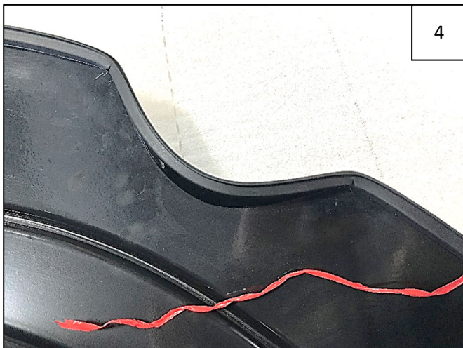
Correctly-installed edge trim around gas door.
