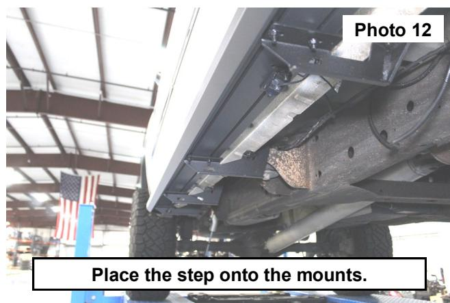
11. Center the step to the body of the vehicle and tighten all step hardware. **See Photos 13 and 14.**
