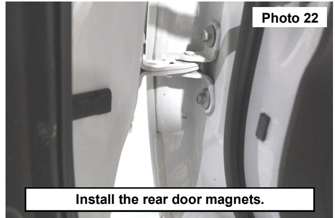
20. Align the door magnet with the rear sensor. **Notes:** The magnet can be taped onto the door to set the correct placement before the double sided tape is applied. Place the magnet onto the door using the double sided tape on the back of the magnet. **See Photo 22.** Repeat on passengers side.
