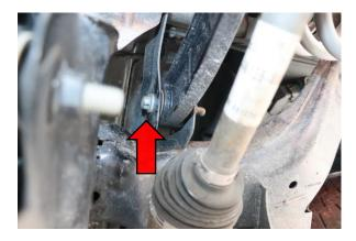
Step 3. Remove and discard the 15mm bolt securing the camber arm to the frame. Remove the OE camber arm from the truck. (Note OE fasteners and torque to yield and one time use)
