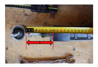
Step 6. Maximum extension of the control arm is 78mm when measured from the bottom of the bushing to the control arm. This provides a positive camber of +2.8° when used with Eibach lift spring.
