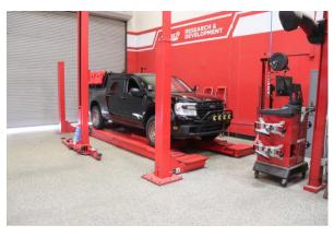
Step 8. Perform an alignment to set all camber and toe angles to manufacturer specification. Test drive vehicle to ensure correct alignment.
