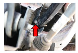
Step 5. Install **new** 15mm bolt securing the camber arm to the frame (some force may need to be used to align the camber arm with the frame mounting point). Tighten both 15mm bolts in two stages.
