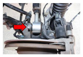
Step 2. Remove and discard the 15mm bolt securing the camber arm to the hub carrier.
