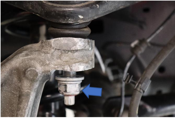
Step 4. Loosen the upper ball joint nut, but do not remove all the way.
