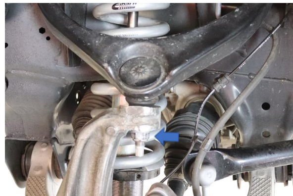
Step 22b. (Torque nut to 26 Ft. Lbs. + 180°)
