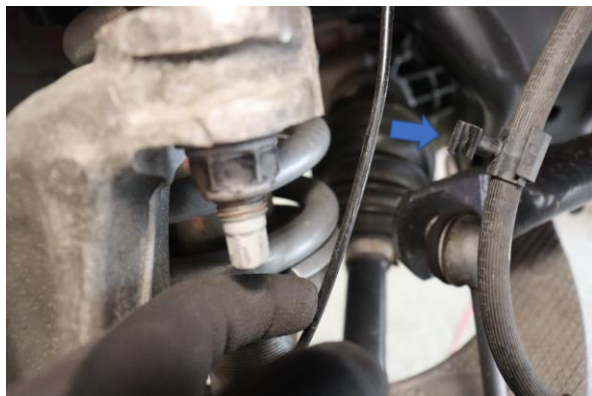
Step 23. Reattach the speed sensor wire to the brake line clip.
