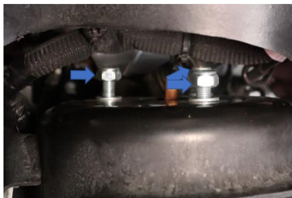
Step 17. Install the 3 flange nuts provided with the kit on top of the shock tower. Torque nuts to 35 Ft. Lbs.
