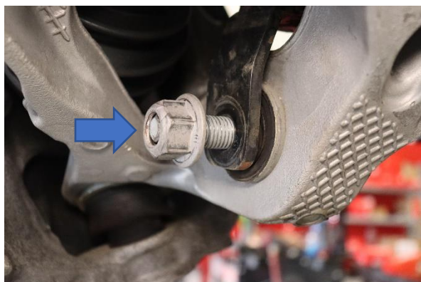
Step 10. Loosen the shock assembly lower nut.
