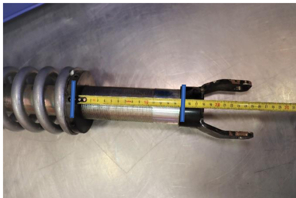
Step 15. Verify the collar height, it is preset to 132mm (5 3/16").
