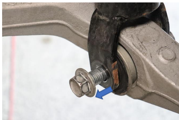
Step 11. Remove the shock assembly lower bolt.
