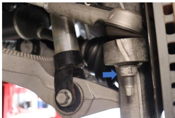
Step 21b. (Torque nut to 38 Ft. Lbs. + 195°)
