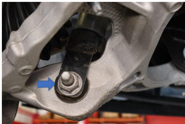
Step 19b. (Torque nut to 124 Ft. Lbs.)
