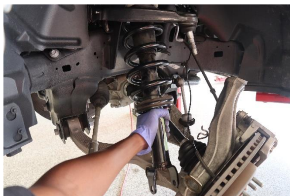
Step 14b. Note: Ensure knuckle does not pull on the brake line, or that it is not pulling on the axle. Tie strap the knuckle to frame if necessary.
