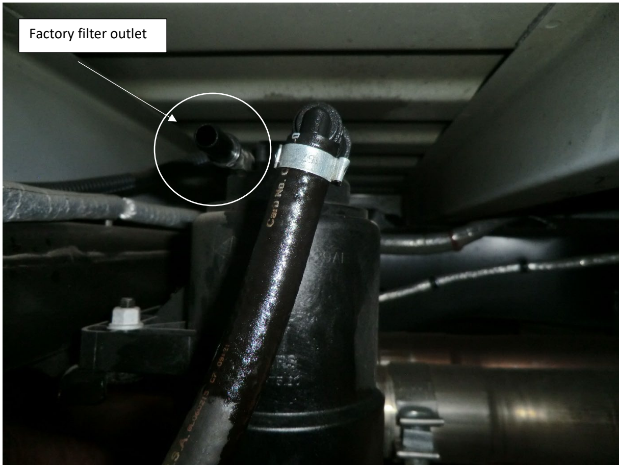
Engine fuel supply line shown in Photo above.
