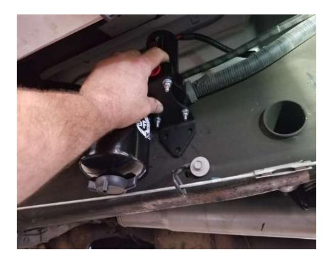
4. Place the fuel manifold assembly on to the truck and mark the three holes using the carbon steel frame bracket.
