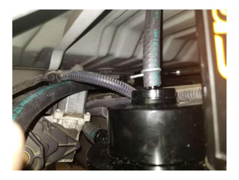
16. Carefully route the ¼" hose to the top of the air chamber on the fuel manifold assembly, making sure not to kink the hose or allow it near moving parts. Carefully mark and then cut the hose to the correct length. Using the supplied spring clamp, attach the hose to the nipple on the top of the air chamber on the fuel manifold assembly.
