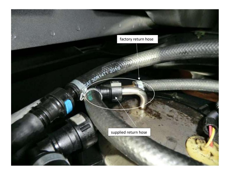
15. Disconnect the factory fuel return line. Attach the supplied fuel return hose between the male and female factory fuel fittings. Push all connections togethers.
