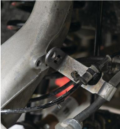
Fig. 1: Brake line bracket.
