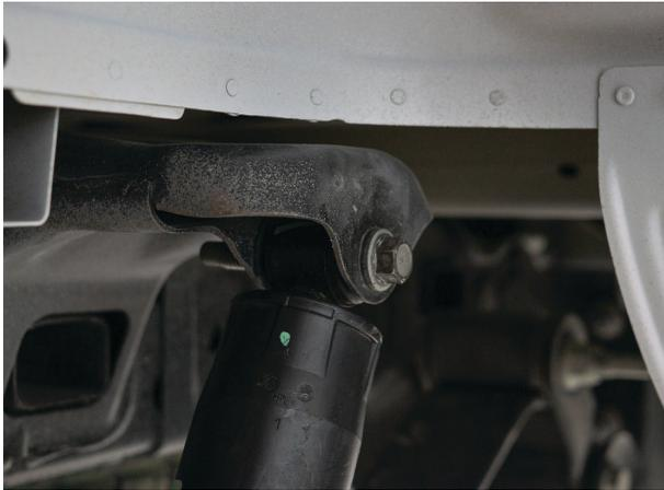
Fig. 19: Remove upper shock mount bolt.
