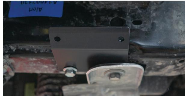
Fig. 9: Install the reservoir bracket.
