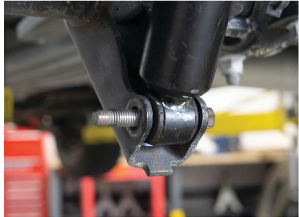
Fig. 20: Remove lower shock mount bolt.
