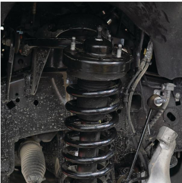
Fig. 6: Free the coil-over.
