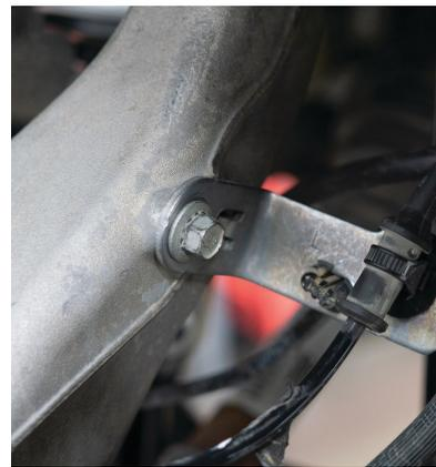
Fig. 18: Brake line bracket.
