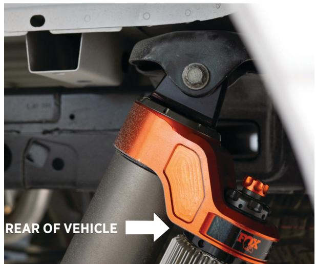
Fig. 21: Install the upper shock mount.
