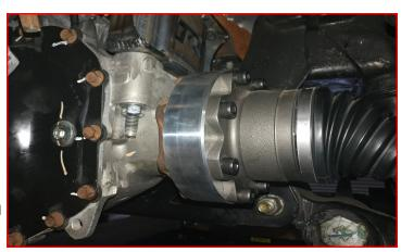
Install the ReadyLIFT passenger side CV (1" thick) spacer in between the CV flange and differential flange using the provided M10 x 50mm Allen bolts, washers and a drop of thread locker. Make sure to line up the previous marks on the flanges. Torque all CV bolts to 50 ft-lbs.
