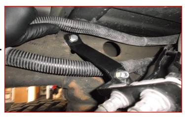
Install the wheels. Torque the lug nuts to the wheel manufacturers specs. Torque the upper and lower shock mount to 60 ft-lbs, and u-bolt hardware to 120 ft-lbs. Reattach the vehicle power source at the ground terminal.
