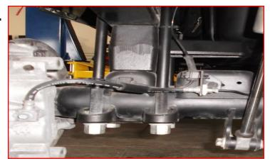
Install the supplied shocks to the frame using the factory hardware.
