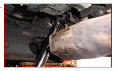
Once the cross member is removed, pull the torsion bars out of the lower control arms and set aside. Make sure to have the bars marked for reassembly. It is best to lay the bars down on the ground under the vehicle in the same orientation/side as they are removed.
