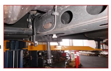
Add pressure by tightening the forcing screw to the torsion bar until there is enough room to remove the torsion bar adjustment pin from the cross member. Once the pin is removed, release the pressure on the torsion bar by loosening the forcing screw. Repeat for both sides.
