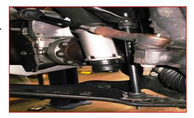
Install the provided shocks to the frame using the provided hardware that came with the shocks.
