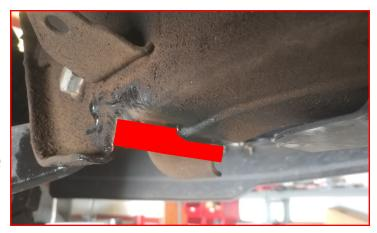
Install the ReadyLIFT passenger side diff drop to the original hanger using the provided M12 nuts and washers. Install the differential to the hanger using the provided M12 bolts, washers and factory nuts. Do not tighten at this time.
