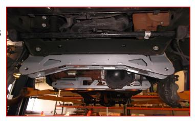
Install the lower control arms to the ReadyLIFT cross members using M18 bolts, washers, and nuts. Do not tighten at this time. If you are installing the 7-8" lift kit, Install the ReadyLIFT upper control arms now.
