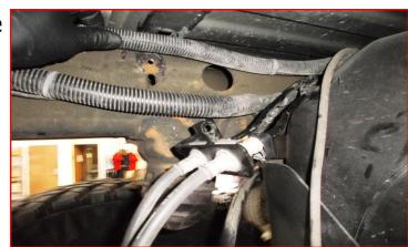
Locate the parking brake cable at the frame rail ahead of the driver side leaf spring mount. Pull on the cable and pop the adjuster out of the cable clamp. Pull the driver side cable out of the frame rail. Reposition under the leaf spring mount and reinstall to the original holes. Push the cable until the clips lock into place. Install the cable end back into the cable clamp.
