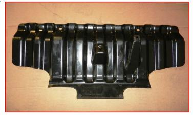
Install the gravel guard between the ReadyLIFT cross member and the factory cross member. As you raise the guard to the core support bar, make sure to guide the lower radiator hose clamp into the guard mounting hole. Press into place. Install the front edge to the factory core support bar using the factory hardware. Tighten down by hand. Install the wheels and lower the vehicle to the ground. Torque the lug nuts to the wheel manufacturers specs.
