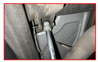
Install the supplied shocks to the axle using the factory hardware.
