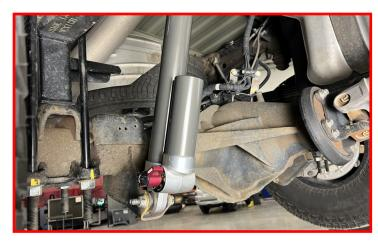
Install the ReadyLIFT brake line bracket to the frame and metal factory bracket using the factory hardware and 1/4" bolt, washer and nuts. Torque to 5 ft-lbs. Reconnect ABS electrical connectors. Make sure there is enough slack for full droop, adjust as necessary. Zip tie to ubolts at full droop.
