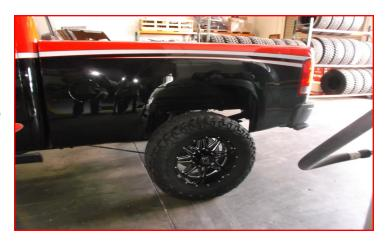
Move to the front of the truck. Set the ride height of the vehicle by measuring from the center of the wheel to the fender edge straight above. Make sure that if you have deep dish wheels, that you use a straight edge and level to find center of the wheel and straight edge at the fender. DO NOT measure by going around the lip of the wheel. Use of a straight edge and level may be necessary for deep dish wheels.
