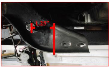
Using a suitable cutting tool, cut along the previous made marks. Remove and discard the outer portion of the control arm pocket. Paint the exposed metal with a quality rust preventative paint.
