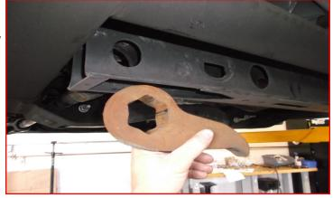
With the torsion bar slid forward, remove any wire harness that is attached to the cross member. Remove the torsion bar cross member from the frame.
