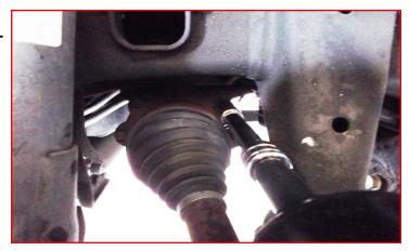
Remove the CV axle from the vehicle.
