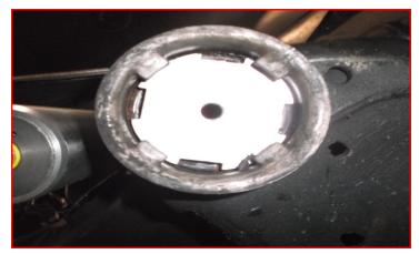
Install the ReadyLIFT bump stop extension using provided 3/8" x 5.5" long Allen head bolt and washer. Torque to 35 ft-lbs.
