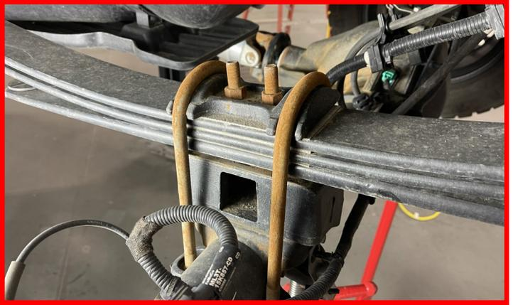
**Remove the driver side u-bolts completely and discard.**
