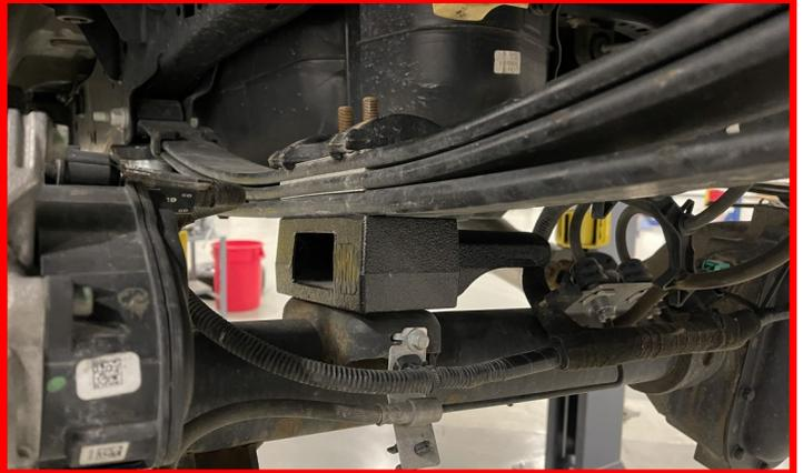
Install the provided u-bolts, and nuts. Snug the u-bolt nuts but do not fully tighten at this time.
