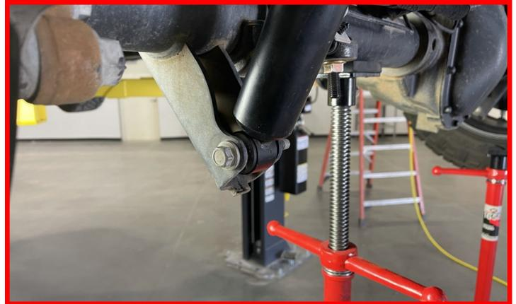
Remove the rear sensor bracket from the forward axle center pin.
