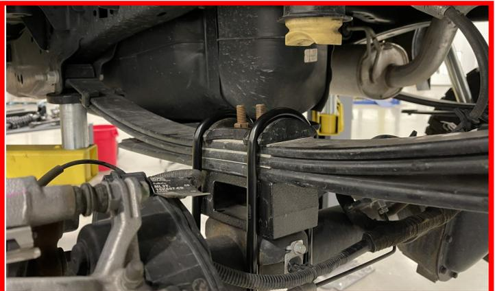
Install the rear sensor bracket on the forward axle center pin in the factory orientation.
