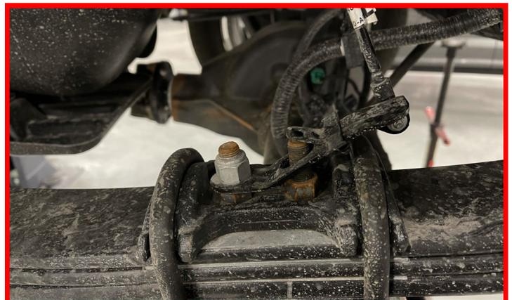
Slightly loosen but do not remove the Passenger side u-bolts.
