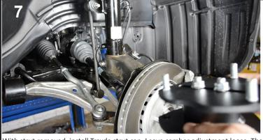
With strut removed, install Traxda strut cap. Leave camber adjustment loose. The arrow on part faces forward. Right and left sides of truck use the same part.
