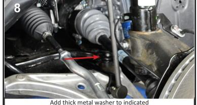
bolt to create space between bolt and axle.
