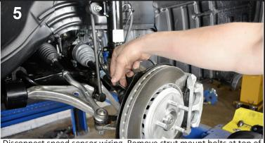
Disconnect speed sensor wiring. Remove strut mount bolts at top of strut, behind plastic cover. Remove lower strut mount bolt.
