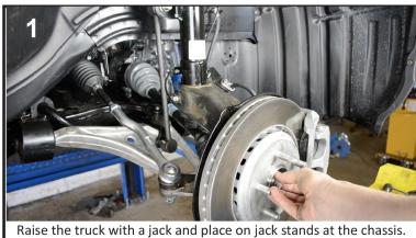
Remove wheels and tires. REMOVE AXLE NUT
