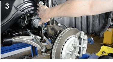
Remove sway bar links and ball joint.
