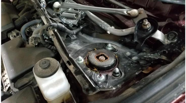
8. Place Traxda part on strut and bolt on
