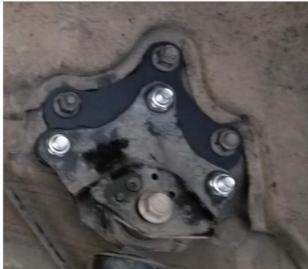
10. Re install spring and reattach control arm bolt
