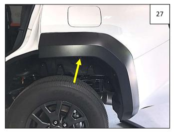
Start one supplied 20mm Hex Screw through flare and into #14 "U" Clip installed in Step 25 (indicated by arrow).
