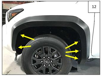
Install 5 supplied 20mm Hex Screws through remaining holes in flare and into holes in fender. Do not tighten.
