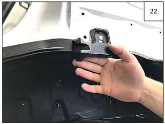
Slide a supplied Long "U" Clip over mark made in Steps 20-21, making edge of clip flush with outer edge of wheel well lip as shown.
