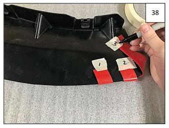
Use masking tape to hold each tape leader in place. Use a sharpie to number each tape piece as shown.
