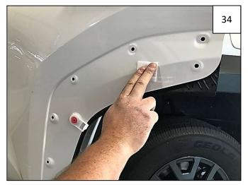
Use a supplied Alcohol Wipe to thoroughly clean the door where the Door Piece will be installed. Surface must be free of grease and dirt.
