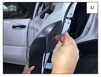
Hold Outer Door Piece in place over Inner Door Piece. Start 3 supplied #10 Truss-Head Screws through Outer Door Piece and into clips installed in Inner Door Piece in Steps 35-36.
