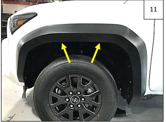
Aligning flare on fender and pressing toward vehicle, start 2 supplied 20mm Hex Screws through flare and into clips installed on Inner Bracket. Do not tighten.
