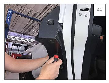
Apply pressure to Door towards vehicle body at each fastening point and tighten all fasteners.
