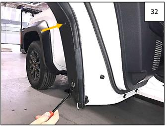
With door open, use a pry tool to remove 2 factory plastic retainers located along edge of flare.
