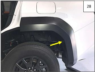
Start one 20mm Hex Screw through hole indicated by arrow and directly into fender.
