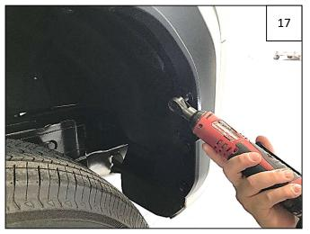
Use a 10mm socket to remove 1 factory bolt indicated by arrow.
