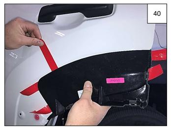
Keeping part snug against door, carefully peel each tape leader starting with the leader marked #1. Peel at a 45-degree angle away from the part to release from the tape, pressing against the part as you go.
