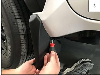
Remove 1 factory screw from underside of mudflap.
