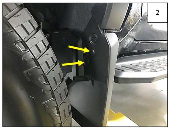
If factory mudflap is present, remove 2 factory screws indicated by arrows.
