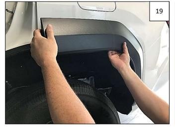
Open the rear passenger door. Pull factory flare away from vehicle, disengaging internal clips. Discard flare, clips, and factory hardware.
