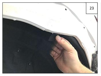
Install a supplied Mylar Tab over metal tab in fender, centering over hole.
