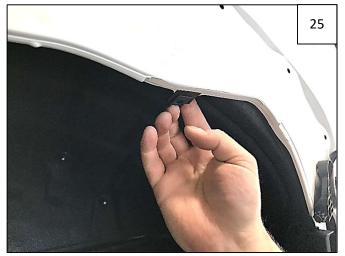
Install a supplied #14 "U" Clip over Mylar Tab Installed in Step 23.
