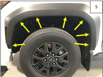
Use a 10mm socket to remove 7 factory screws from wheel well as indicated by arrows.
