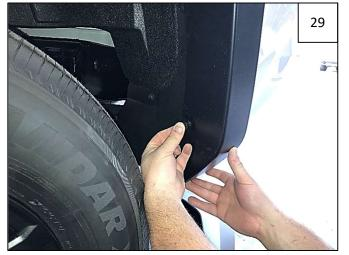
Install a supplied Christmas Tree Fastener through lower rearmost hole in flare and into fender.
