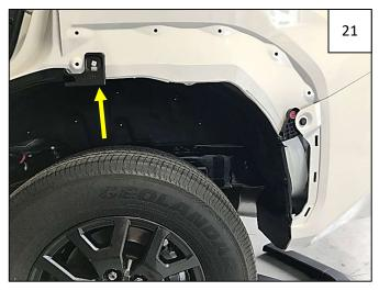
Long "U" Clip location (vehicle with factory flare removed shown, but location is same for both).
