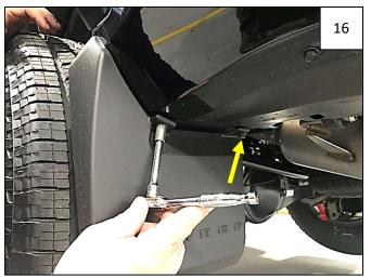
Using a 10mm socket, remove 2 factory screws from underside of mudflap at rear. Remove and discard mudflap.
