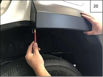
Align flare firmly on fender and use a grease pencil to mark 1 Long "U" Clip location as shown.
