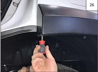
Align flare on fender and start one supplied #10 Truss Head Screw through forwardmost hole and into Long "U" Clip installed in Step 22. Do not tighten.
