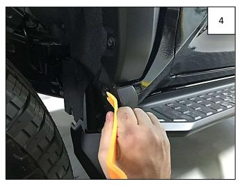
Use a pry tool to disengage plastic clip in wheel well. Remove and discard mudflap.
