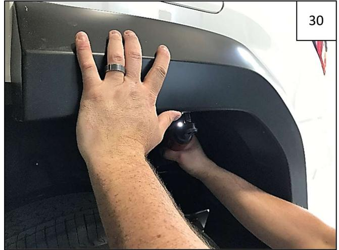
30 Apply pressure to flare towards vehicle body at each fastening point and tighten all fasteners.
