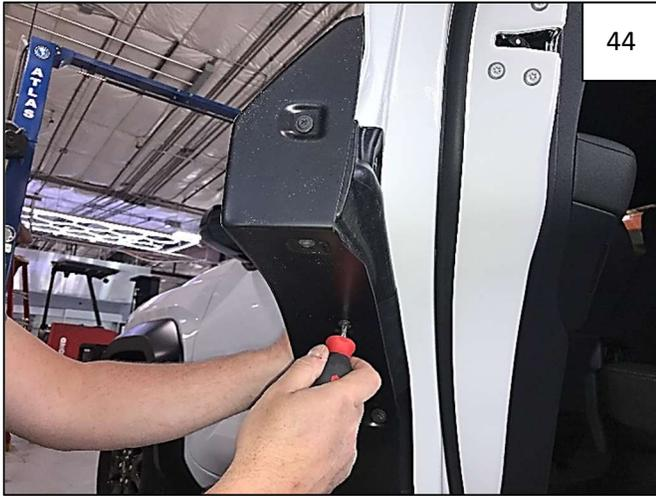
Apply pressure to Door towards vehicle body at each fastening point and tighten all fasteners.
