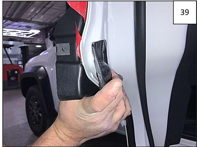
Place Inner Door Piece snugly against door, aligning formed-in feature of part with edge of door as shown. Make sure the red tape leaders are accessible.
