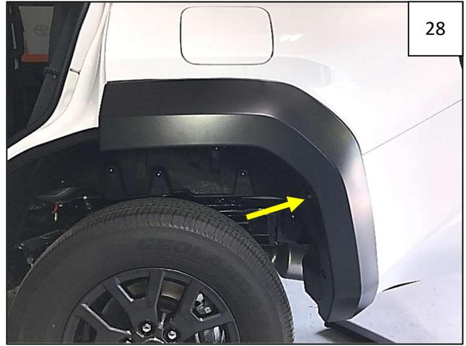
28 Start one 20mm Hex Screw through hole indicated by arrow and directly into fender.
