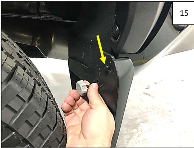
If factory mudflap is present, use a #2 Phillips screwdriver to remove 2 factory screws indicated by arrows.
