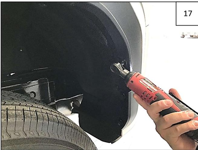
Use a 10mm socket to remove 1 factory bolt indicated by arrow.
