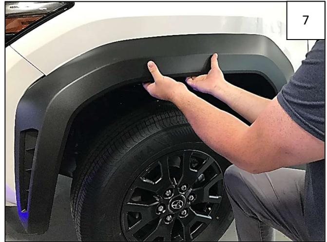
Pull factory flare away from vehicle, disengaging internal clips. Discard flare, clips and factory hardware.
