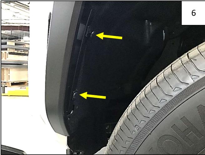
Use a pry tool to remove 2 plastic clips.
