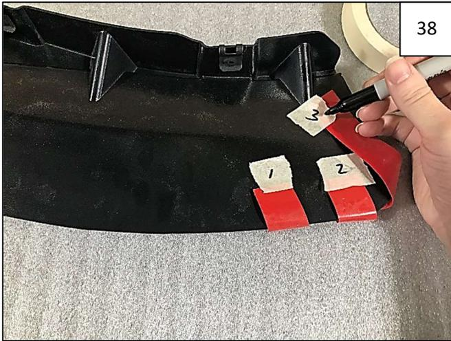
Use masking tape to hold each tape leader in place. Use a sharpie to number each tape piece as shown.
