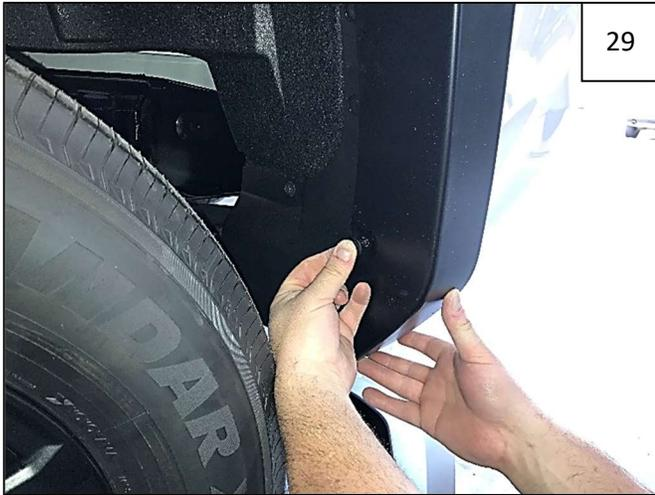
29 Install a supplied Christmas Tree Fastener through lower rearmost hole in flare and into fender.
