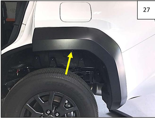
27 Start one supplied 20mm Hex Screw through flare and into #14 "U" Clip installed in Step 25 (indicated by arrow).
