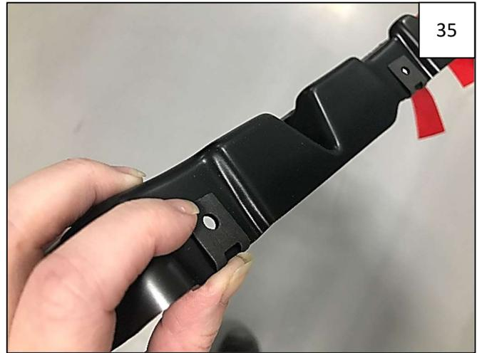
Install 3 supplied #10 "U" Clips onto Inner Door Piece as shown. Flat side of clip will face out.
