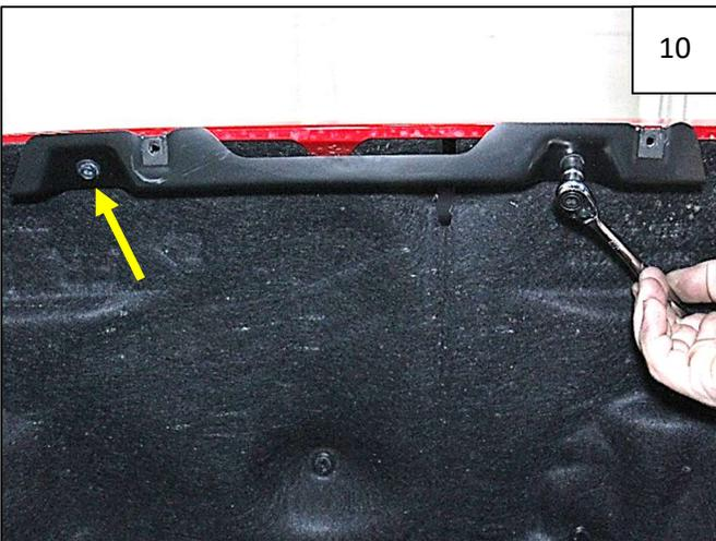
Align holes in Inner Bracket with uppermost holes in fender. Start 2 supplied 20mm Hex Screws through Inner Bracket and into holes in fender. Tighten screws.
