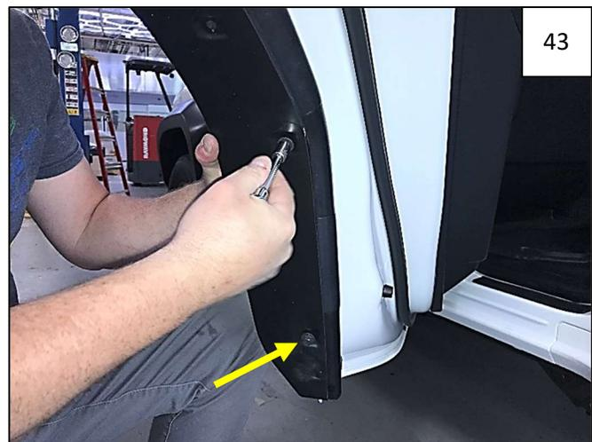
Start 2 supplied 20mm Hex Screws through lower holes in Outer Door Piece and into Door.
