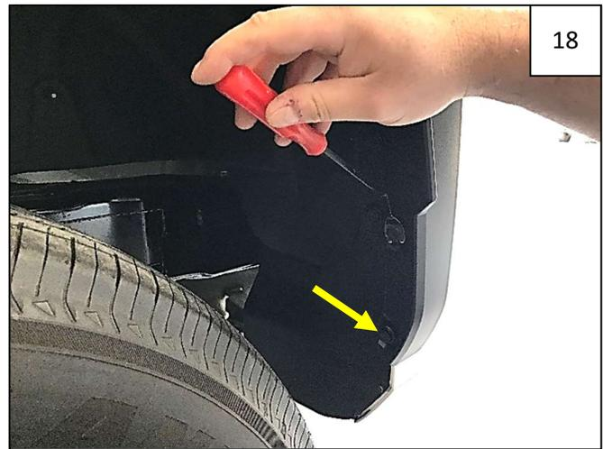
Use a pry tool to remove 2 plastic retainers below bolt removed in Step 18.
