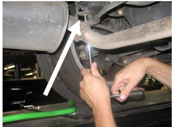
8. Position your new ST Anti-Sway Bar on the vehicle, (photo 4), install the O.E. end link, but do not totally tighten, to one of the holes on the end of the Anti-Sway Bar. Use the same hole on each side.
