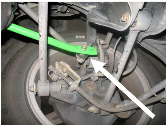
9. Thoroughly lubricate the **inside** of your new bushings using the supplied grease. Place the bushing on the new Anti-Sway Bar. Refer to the original equipment Anti-Sway Bar as to the proper bushing location.
