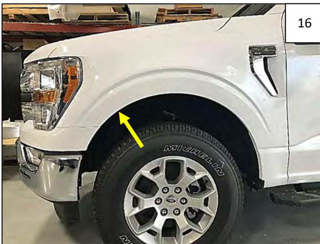
Using a 7mm socket, reinstall 1 factory screw through the Inner Bracket and into fender.
