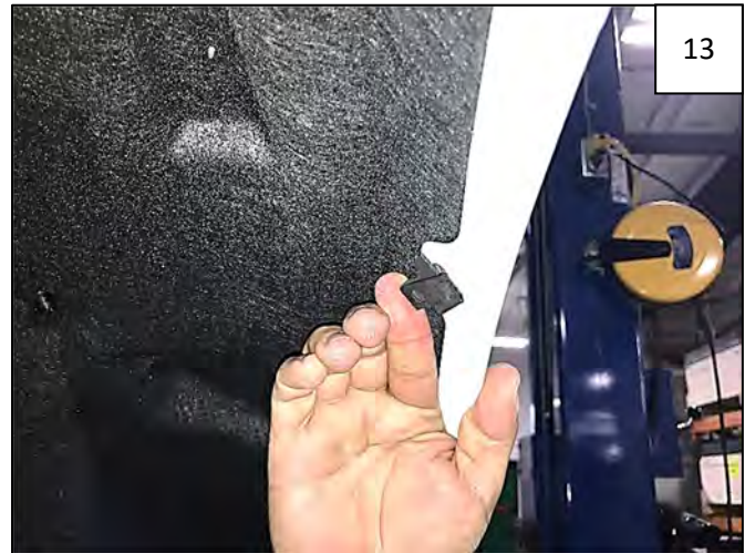
Slide a supplied Long "U" Clip over each Foam Tab installed in Step 11.
