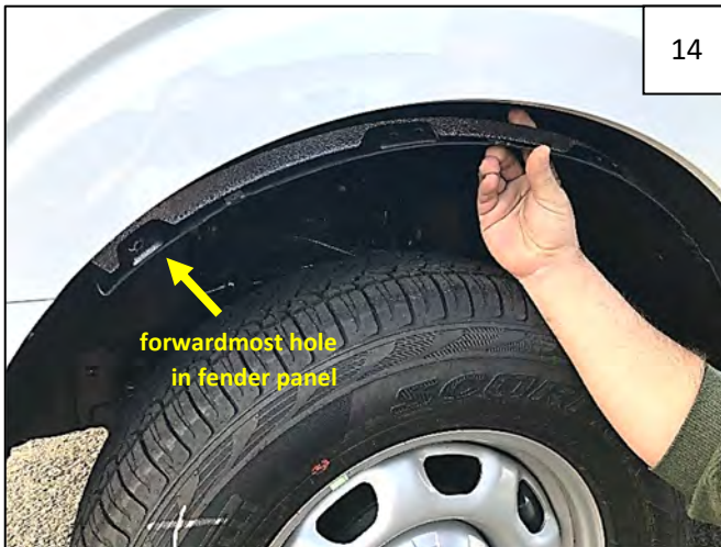
Line up Inner Bracket holes shown in Step 18 starting with the forwardmost hole in the fender panel and continuing with clips installed in Step 13. Inner Bracket will follow the curvature of the wheel well.
