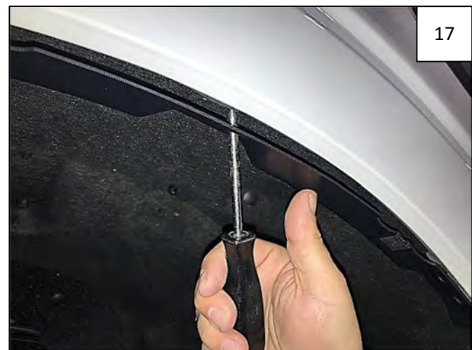
Use an awl to locate holes in clips for ease of screw installation in next step.
