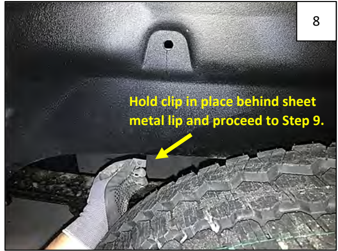
8 Hold a supplied "U" Clip behind wheel well liner and sheet metal at back front of rear wheel well – this Clip will not fit over the lip in the sheet metal and must be held in place until the Bolt is engaged in Step 9. Flat side of clip will face toward you.
