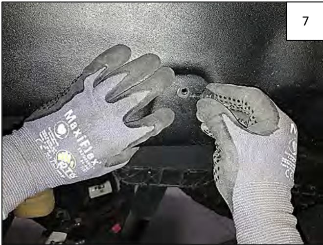
7 Start a supplied 10mm Bolt through hole in back rear of wheel well liner and into clip installed in Step 3. Tighten bolt.
