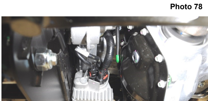
Plug in rack and pinion and diff actuator.
