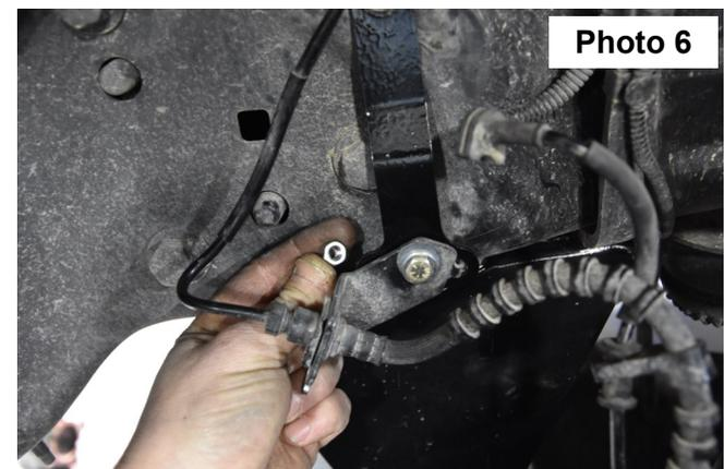
10. Using 18mm and 15mm wrenches, remove the factory steering stabilizer from the truck.
