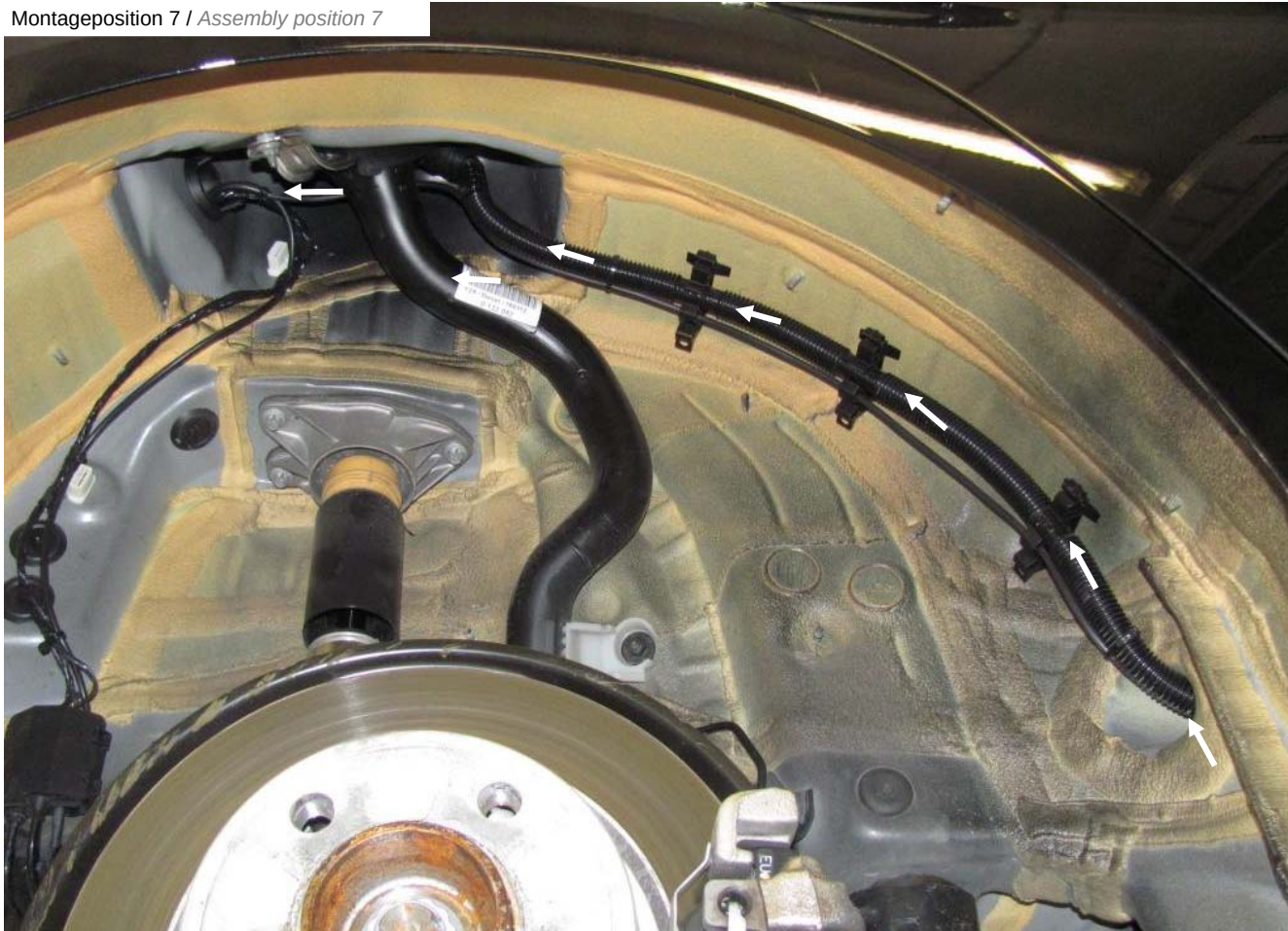
Montageposition 7 / Assembly position 7
