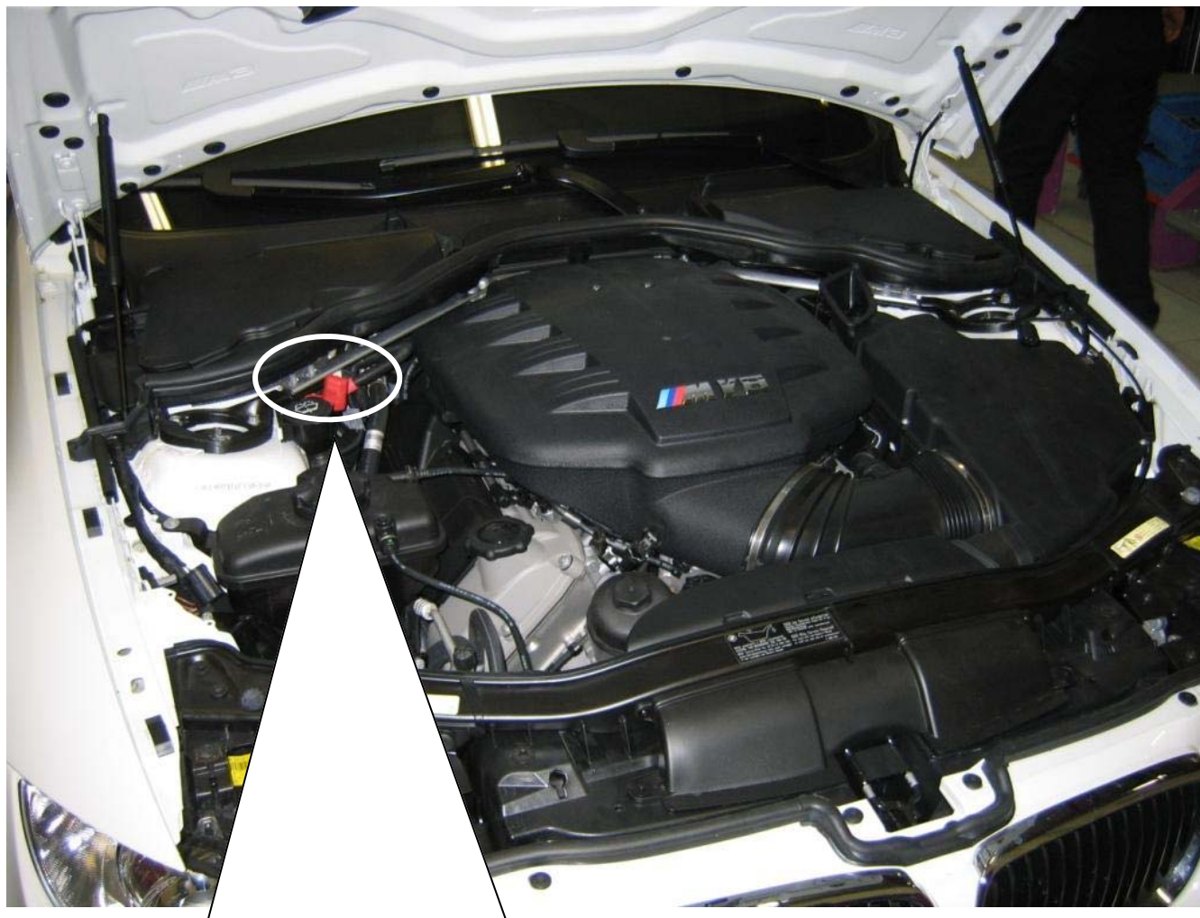
Montageort VA Elektroniksatz / Assembly area front axle electronic kit
