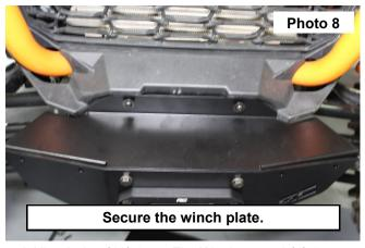
10. Secure the cover plate using (6) 6mm-1.0 x 20mm button head Allen bolts, (10) 6mm Flat Washers and (4) 6mm—1.0 Nylock Nuts. Place (2) bolts in the center top of the cover and (2) bolts and nuts in each side of the winch plate. **See Photos 9 and 10.** Tighten using a 4mm Allen wrench and a 10mm wrench.
