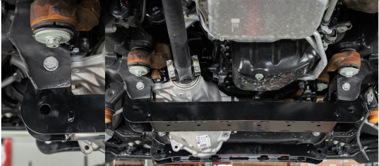
Figure 38: Install Rear Crossmember
