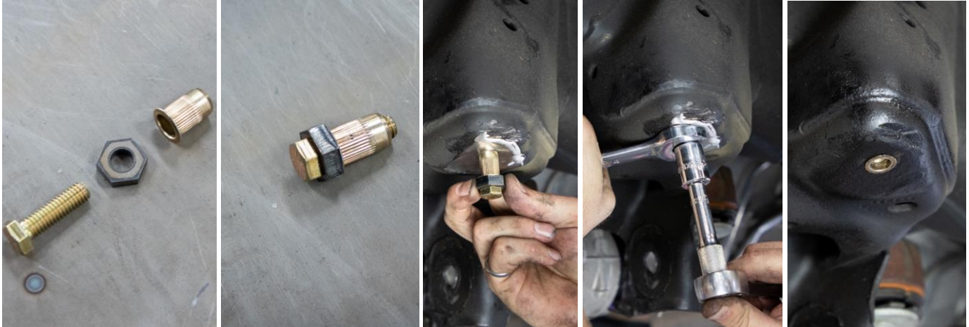
Figure 33: Install Tool for Rivet Nut
