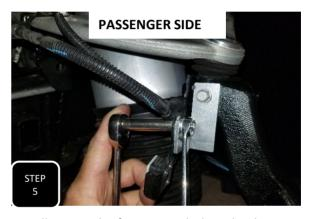
**Step 5** Attach the provided 1019AR-P bracket to the neck of the spindle using the factory M6 bolt and tighten. Next, attach the factory body position sensor to the bracket using the provided M6 bolt, nut & washers, then tighten.
