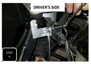
**Step 4** Models with air ride will attach the provided 1019AR-D bracket to the neck of the spindle using the factory M6 bolt and tighten. Next, attach the factory body position sensor to the bracket using the provided M6 bolt, nut & washers, then tighten.
