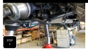
Step 1 Unbolt the sway bar end link from the control arm on both sides
