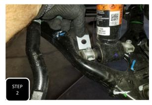
**Step 2** Unbolt the two bolts attaching the strut to the lower control arm and then insert the provided 1019AR-1 spacer plates between the strut's barpin and the control arm.
