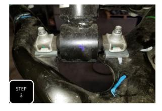
**Step 3** Once both spacers are in place then re-install the factory bolts and tighten to 40 ft/lbs.
