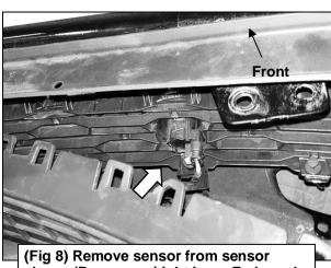
sleeve (Passenger/right inner Z-shaped sensor pictured from behind bumper)
