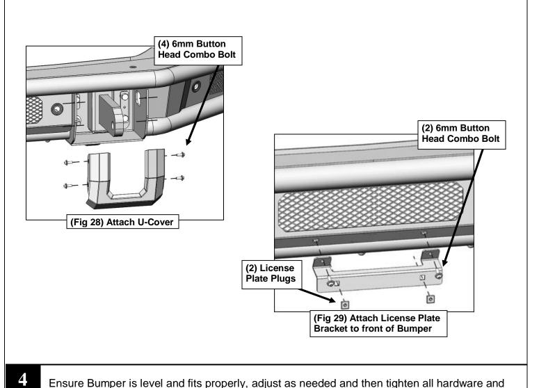
Ensure Bumper is level and fits properly, adjust as needed and then tighten all hardware and double check all connections. Installation is complete. Do periodic inspections to the installation to make sure that all hardware is secure and tight.
