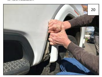
Carefully pry factory flare away from vehicle, starting at lower front or rear and working up to top center, taking care not to break factory clips if possible. Pry any remaining clips from fender using a plastic pry tool.
