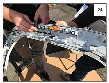
Reroute wire harness in factory flare. **NOTE:** <u>Make sure light connector is pulled through factory flare and accessible for reconnection.</u>
