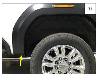
Still holding flare firmly on fender, start 1 factory fastener at underside front of flare at location shown.
