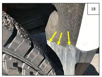
Remove 3 T-15 Torx screws from rear mud guard at inside rear of wheel well. Retain all screws. **NOTE:** Some screws will be used for flare installation.
