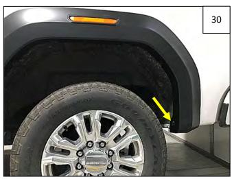
Holding flare firmly on fender, start 1 factory fastener through rearwardmost hole in flare and into fender at location shown.
