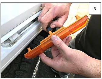
Disconnect side marker light from wire harness, leaving wire harness connector accessible for reinstallation.
