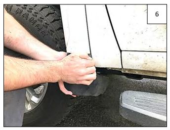
Remove mud guard by prying down and away from vehicle body, disengaging one internal clip. Discard mud guard.
