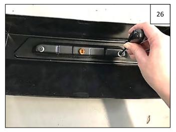
Install side marker light into fender flare using 2 supplied nylon spacers and screws retained in Step 22. Before tightening, check alignment of light in light pocket. Do not overtighten screws.
