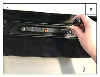
Install side marker light into fender flare using 2 supplied nylon spacers and screws retained in Step 2. Before tightening, check alignment of light in light pocket. Do not overtighten screws.
