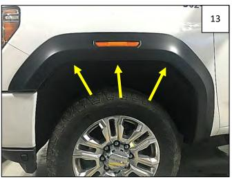
Start 3 supplied #10 Short Truss-Head Screws through holes in flare and into clips installed in Step 12. **NOTE:** Clip locations may be adjusted by hand and/or an awl may be used to align holes prior to screw installation.
