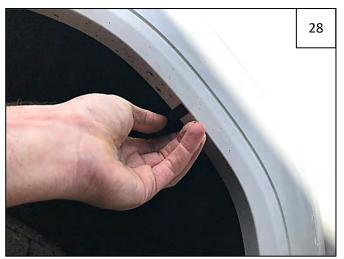
Remove flare from fender and slide a supplied #10 "U" Clip flat-side down over each mark made in Step 27, centering on mark and aligning edge of clip with edge of fender lip. Clip holes should be free of interference.
