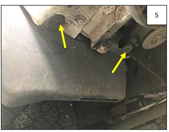
Remove 2 T-15 Torx screws from underside of mud guard.
