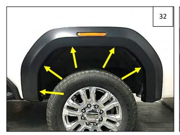
Start 5 supplied #10 Long Truss-Head Screws through holes in flare and into clips installed in Step 28. **NOTE:** Clip locations may be adjusted by hand and/or an awl may be used to align holes prior to screw installation.
