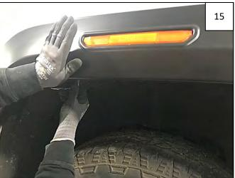
Ensure flare fit. Apply pressure to outward face of the flare towards the center of the vehicle and tighten all screws.
