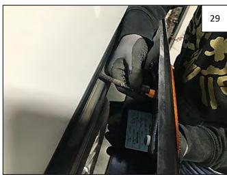
Reconnect side marker light to wire harness before installing fender flare.
