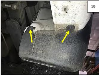
Remove 2 T-15 Torx screws from underside of rear mud guard. Disengage metal clip and remove and discard mud guard.
