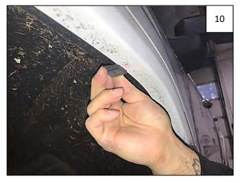
Remove flare from fender and slide a supplied #10 "S" Clip holeside down over each mark made in Step 19, centering on mark and aligning edge of clip with edge of fender lip. Clip holes should be free of interference.
