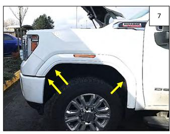
Remove 3 T-15 Torx screws from inside wheel well at locations shown.
