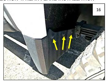
Remove 3 T-15 Torx screws from front mud guard at inside front of wheel well. Retain all screws. **NOTE:** Some screws will be used for flare installation.
