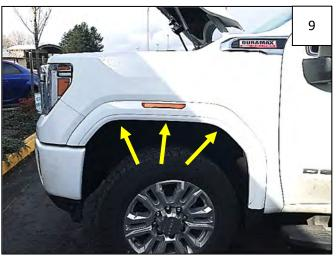
Hold flare firmly on vehicle. Using a grease pencil, mark 3 clip locations at locations shown. **NOTE:** it may be helpful to loosely install 2 factory screws in lowermost flare holes prior to this step for added stability.
