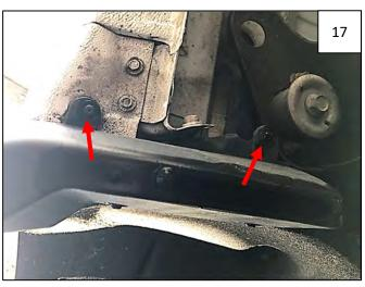
Remove 2 T-15 Torx screws from underside of front mud guard. Disengage lower clip and remove and discard mud guard.
