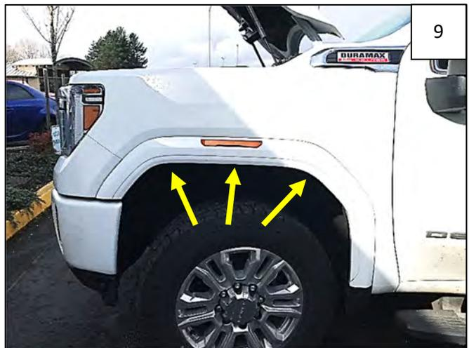
Hold flare firmly on vehicle. Using a grease pencil, mark 3 clip locations at locations shown. **NOTE:** it may be helpful to loosely install 2 factory screws in lowermost flare holes prior to this step for added stability.
