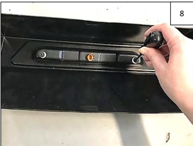
Install side marker light into fender flare using 2 supplied nylon spacers and screws retained in Step 2. Before tightening, check alignment of light in light pocket. Do not overtighten screws.
