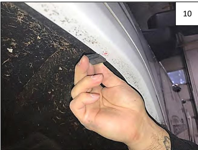
Remove flare from fender and slide a supplied #10 "S" Clip hole-side down over each mark made in Step 19, centering on mark and aligning edge of clip with edge of fender lip. Clip holes should be free of interference.
