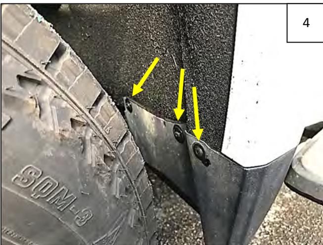
Remove 3 T-15 Torx screws from mud guard at inside rear of wheel well. Retain all screws. **NOTE:** Some screws will be used for flare installation.
