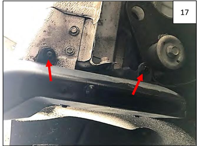
Remove 2 T-15 Torx screws from underside of front mud guard. Disengage lower clip and remove and discard mud guard.
