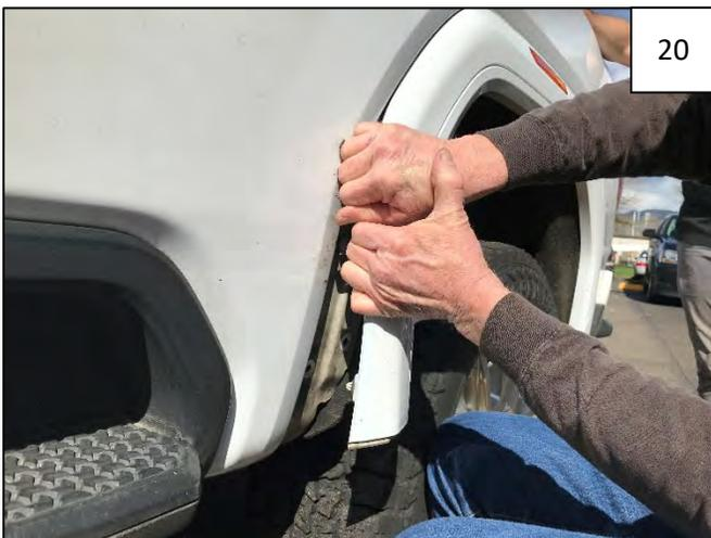
*Carefully* pry factory flare away from vehicle, starting at lower front or rear and working up to top center, taking care not to break factory clips if possible. Pry any remaining clips from fender using a plastic pry tool.
