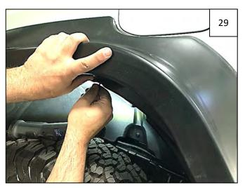
Keeping flare on fender, press inward, firmly with force, on the flare to line up the flare mounting holes with the clips on the Inner Bracket. Install 3 supplied Truss-Head Screws through holes in flare and into clips.
