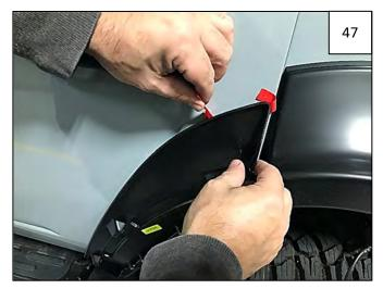
Starting with *lower* tape leader, carefully peel at 45-degree angle away from the part to release from the tape, pressing against the part as you go.
