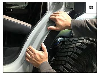
Press part against vehicle at areas of tape for 30 seconds to ensure full adhesion. Tape cures after 24 hours at 65F degrees.
