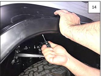
Aligning flare on fender, press inward, firmly with force, on the flare to line up the flare mounting holes with the clips on the Inner Bracket. Install 2 supplied Truss Head Screws through holes in flare and into clips.
