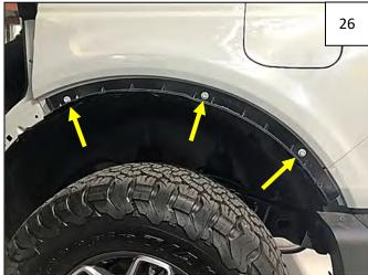
Use factory screws removed in Step 20 to install Rear Inner Bracket, aligning 3 forward-most holes in bracket with holes in fender.
