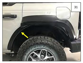
Install a supplied Push-Lock Retainer through hole in flare indicated by arrow and into fender.
