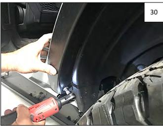
Install 7mm fastener removed in Step 22.
