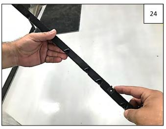
Install 3 supplied "U" Clips onto the Rear Inner Bracket as shown. Note: Driver's side Inner Bracket is marked "LF" and the passenger's side Inner Bracket is marked "RF."
