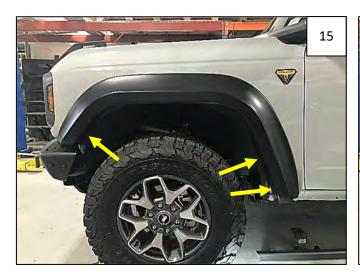
Push 3 supplied Push-Lock Retainers through 3 holes in flare and into fender at areas indicated by arrows.
