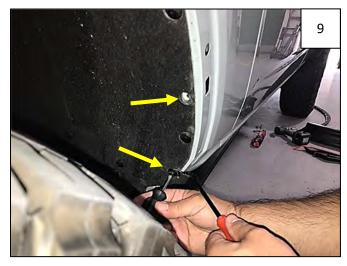
Use a pry tool and Phillips screwdriver to remove 2 plastic retainers at rear of wheel well.
