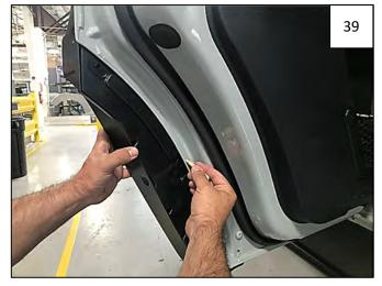
Still carefully holding door piece in position, Using a grease pencil, make 3 marks on edge of door lip aligning with 3 holes in Inner Door Piece.
