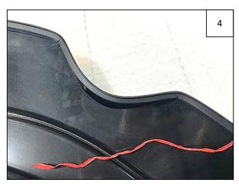
Correctly-installed edge trim around gas door.
