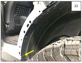
Use a 7mm socket to remove and retain 1 fastener at bottom of door.
