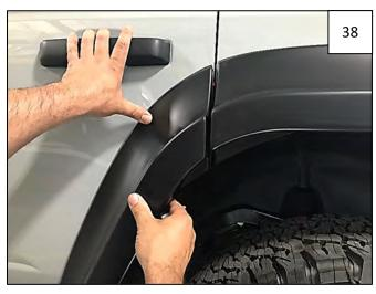
Hold Door Piece combo on (partially closed) door, aligning carefully with rear flare. Taking care to hold Door Piece in place, open door.
