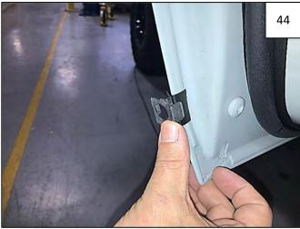
Carefully position a Pinch Clip combo over each Mounting Tab installed in Step 41 – center on the Tab very carefully so the door piece will be aligned properly.
