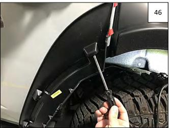
Hold Inner Door Piece on door, keeping red tape leaders free and accessible. Loosely install 3 supplied Truss-Head Screws through Inner Door Piece and into clips on door. Do not tighten.
