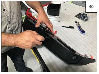
Remove Door Piece combo from door and remove 3 screws installed in Step 37.
