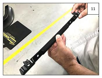
Install 2 "U" Clips onto the Front Inner Bracket as shown. NOTE: Driver's side Inner Bracket is marked "LF" and the Passenger's side Inner Bracket is marked "RF."
