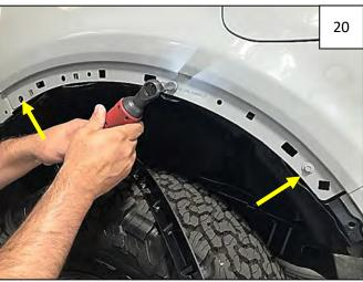
Using a 10mm socket, remove 3 factory screws from fender lip. Retain these screws for installation of the Rear Inner Piece.
