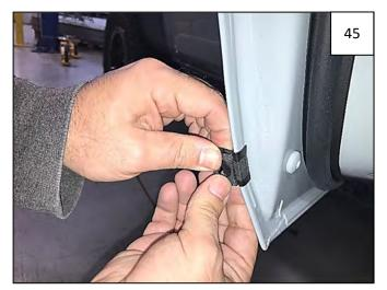
Squeeze the two Pinch Clip pieces shut on door until they snap together. Use a pair of pliers to snap the clips if needed.
