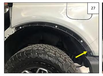
Insert a supplied Christmas Tree Fastener through lower rear 3/8" sized hole in Inner Bracket and into fender.
