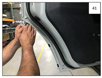
Peel PSA backing from a supplied Mounting Tab. Carefully center a Mounting Tab over each mark made in Step 39, folding tab over door lip.
