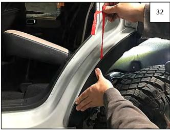
Carefully peel tape leader at 45-degree angle away from the part to release from the tape, pressing against the part as you go.
