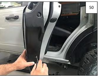
Place Outer Door Piece over Inner Door Piece and reinstall 3 supplied Truss-Head Screws removed in Step 40 as shown.
