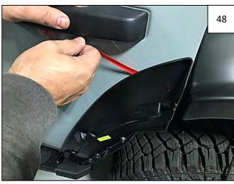
Carefully peel top tape leader at 45-degree angle away from the part. Press part against vehicle at areas of tape for 30 seconds to ensure full adhesion. Tape cures after 24 hours at 65F degrees.
