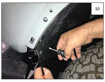
Use a pry tool and Phillips screwdriver to remove 1 plastic retainer at front of wheel well.
