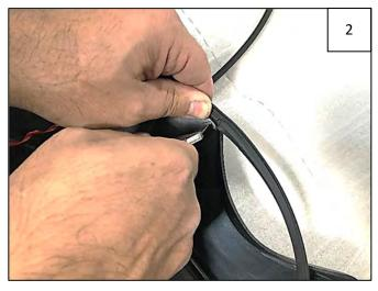
As you come to the first "point" of the flare, cut a "V" notch into the backside of the edge trim at the sharpest part of the curve. Make sure that you retain 2-3 inches of vinyl backing for ease of further installation.
