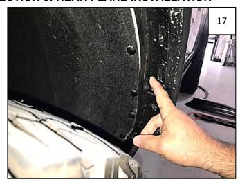
Twist 5 quarter-turn fasteners indicated by arrows, until each fastener disengages.
