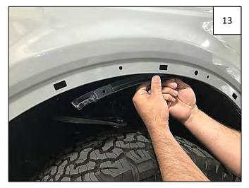
Use factory screws removed in Step 8 to install the Front Inner Bracket, aligning empty holes with holes in fender.
