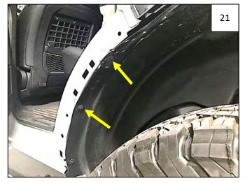
Open the door. Use a pry tool and Phillips screwdriver to remove 2 plastic retainers at front along door seam.
