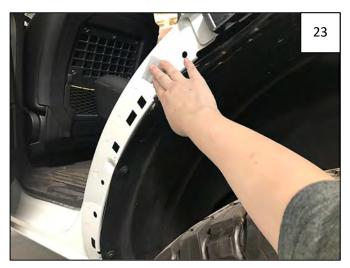
Use a supplied Alcohol Wipe to thoroughly clean dog leg at area of tape. Surface must be free of grease and dirt.
