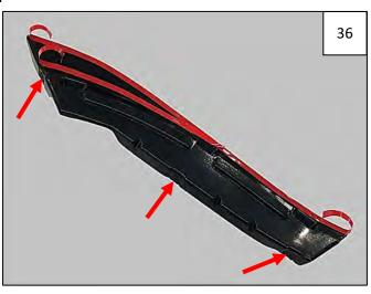
Install 3 supplied "U" Clips onto Inner Door Piece as shown.
