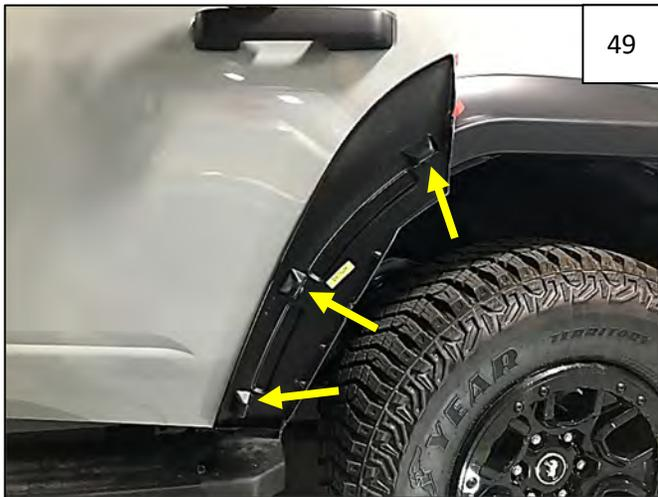
Tighten 3 Truss-Head Screws installed in Step 46.
