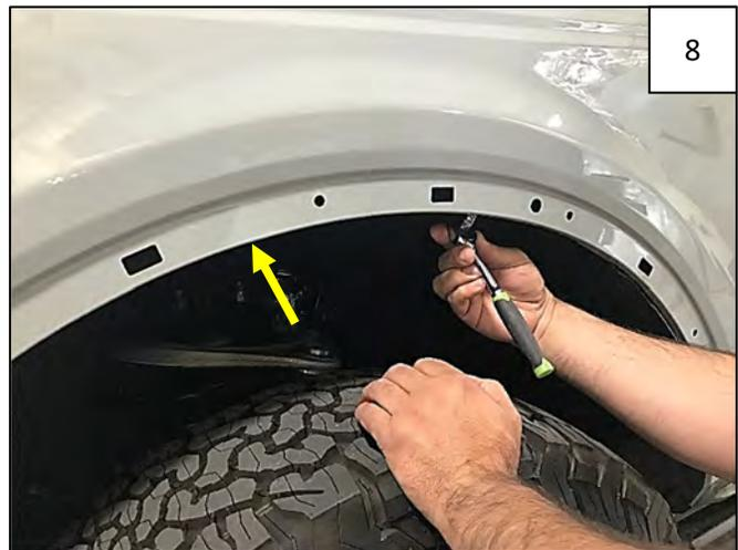
Using a 7mm socket, remove 2 factory screws from inside wheel well. Retain these screws for installation of the Front Inner Piece.
