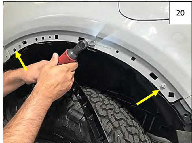
Using a 10mm socket, remove 3 factory screws from fender lip. Retain these screws for installation of the Rear Inner Piece.
