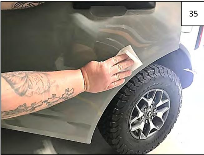
Use a supplied Alcohol Wipe to thoroughly clean the door where the Door Piece will be installed. Surface must be free of grease and dirt.
