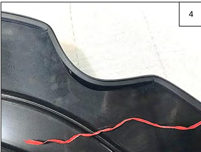
Correctly-installed edge trim around gas door.
