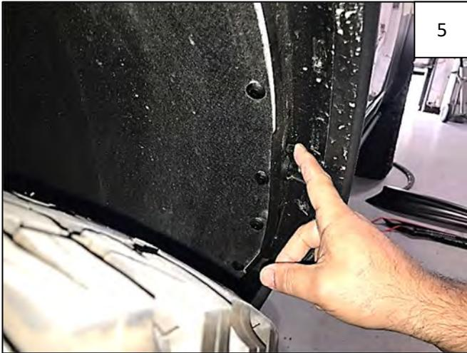
Twist 5 quarter-turn fasteners indicated by arrows, until each fastener disengages.
