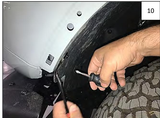
Use a pry tool and Phillips screwdriver to remove 1 plastic retainer at front of wheel well.
