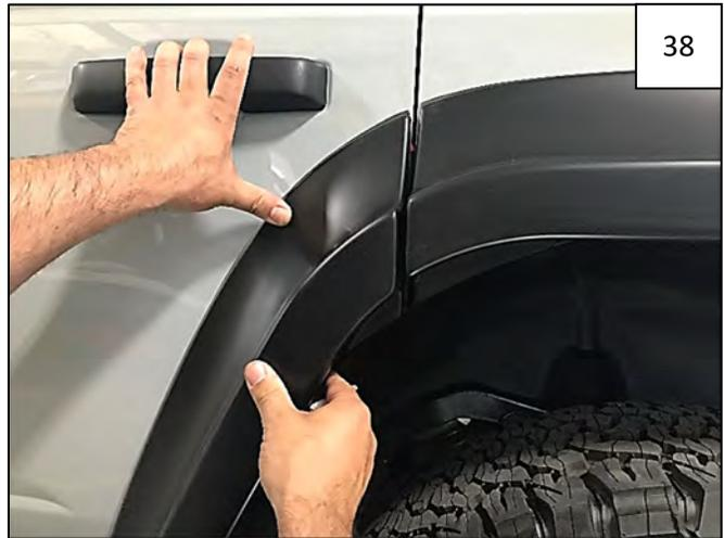
Hold Door Piece combo on (partially closed) door, aligning carefully with rear flare. Taking care to hold Door Piece in place, open door.
