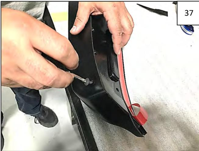
Nest Inner Door Piece into Outer Door Piece, and temporarily install 3 supplied Truss-Head Screws into clips. Install snug but do not tighten, as you will be removing these prior to final installation.
