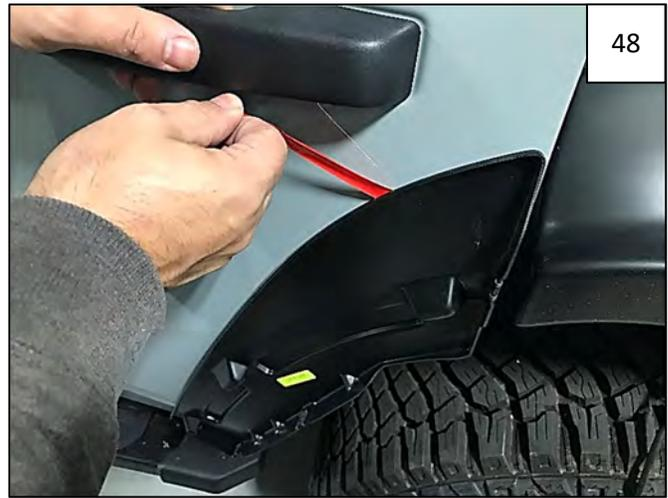
Carefully peel top tape leader at 45-degree angle away from the part. Press part against vehicle at areas of tape for 30 seconds to ensure full adhesion. Tape cures after 24 hours at 65F degrees.
