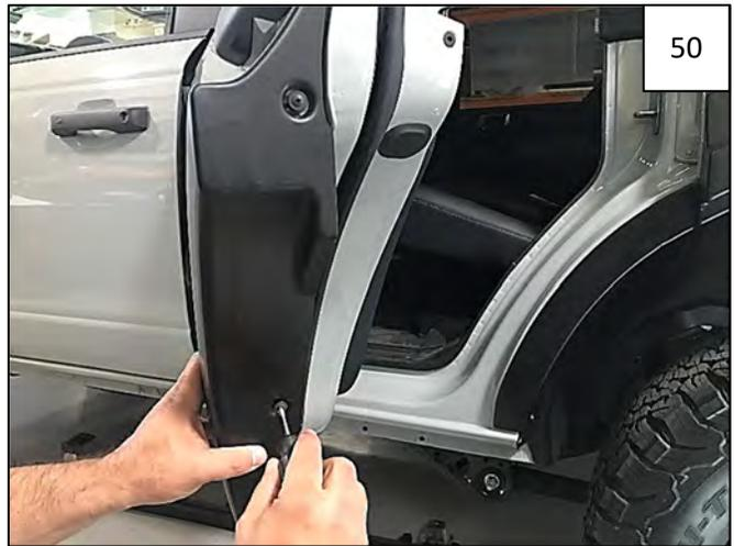
Place Outer Door Piece over Inner Door Piece and reinstall 3 supplied Truss-Head Screws removed in Step 40 as shown.
