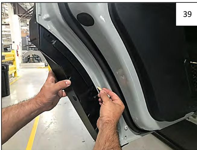
Still carefully holding door piece in position, Using a grease pencil, make 3 marks on edge of door lip aligning with 3 holes in Inner Door Piece.
