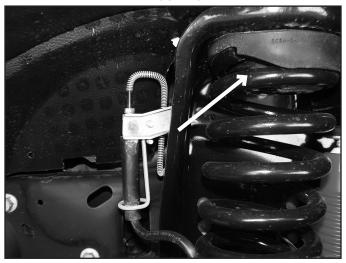
9. Remove the lower coil spring seat from the top of the axle, it will not be reinstalled.
