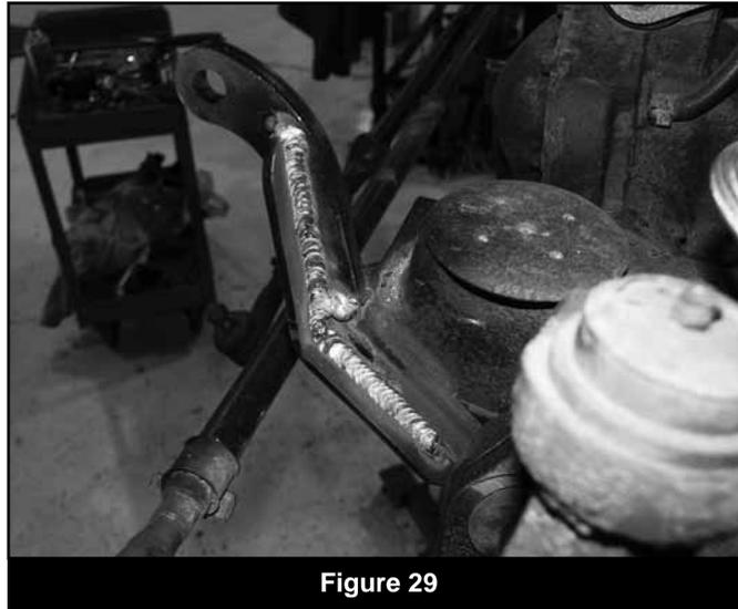
74. With all welding complete allow the brackets to cool and then paint any raw metal to prevent corrosion.
