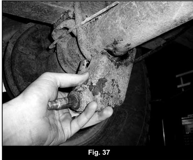
29. Install the new provided shocks to the upper shocks mounts with the original hardware. Torque to 20 ft-lbs. Leave the lower portion of the shock hanging at this time.
