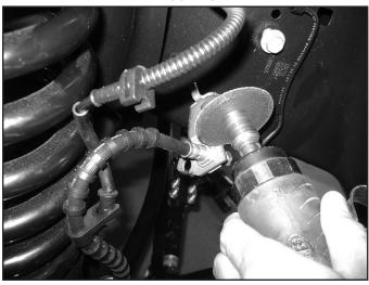
11. Disconnect the shocks by removing factory hardware (Fig 6a, 6b). Retain lower bolt and nut tab for later reinstallation.
