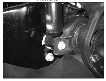
12. Disconnect sway bar from the frame on both the driver and passenger side. Retain (4) mounting nuts. (Fig 7)
