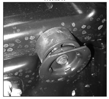
19. Grease the bump stops and reinstall into the factory cups. (Fig 11)
