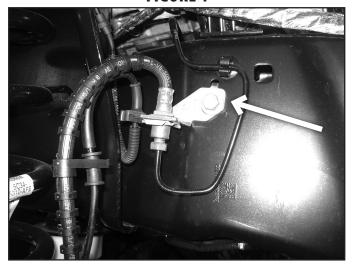
10. Carefully cut the factory bracket so that the brake line can be removed without breaking loose the fittings. Remove the factory brake lines from vehicle. Do not damage the brake line! (Fig. 5)
