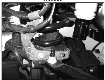
9. Disconnect the brake line bracket on frame (Fig 4). Retain hardware.
