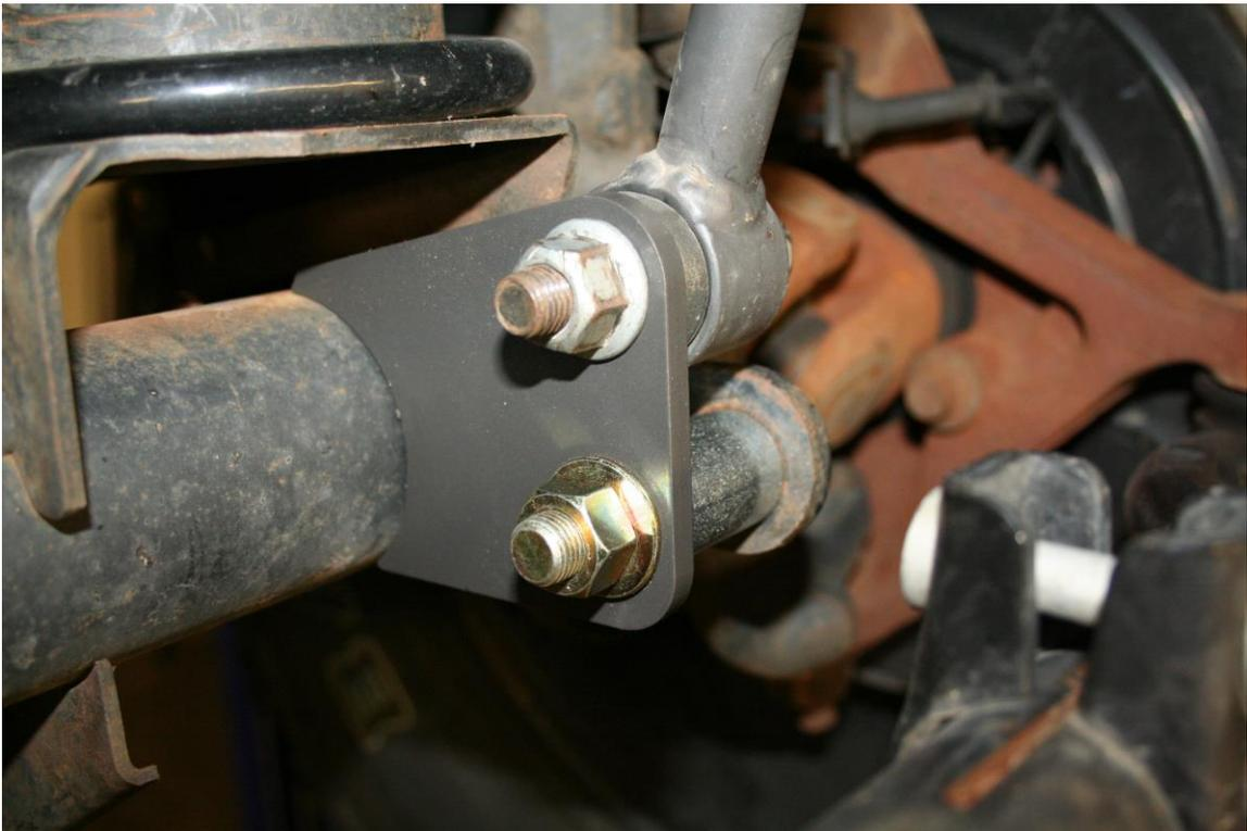
9. If you are not using the anti-sway bar relocation brackets and want to mount the sway bar links in the factory location, install the passenger side anti sway bar link between the track bar bracket and factory sway bar tab as shown below. Attach the driver side anti-sway bar link in the factory location.
