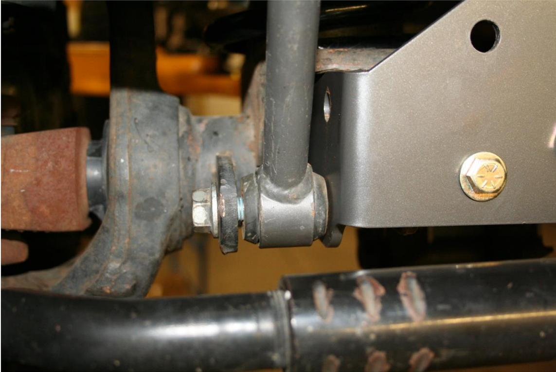
10. The track bar relocation bracket also allows you to relocate the steering stabilizer to the top of the tie rod. Remove the steering stabilizer from the axle bracket and from the tie rod bracket.
