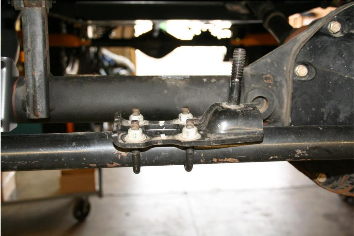
12. Install the steering stabilizer to the tie rod bracket. Attach the shaft end of the steering stabilizer to the track bar relocation bracket using the factory nut and bolt and a  $\frac{1}{2}$  washer between the bushing and the track bar relocation bracket.
