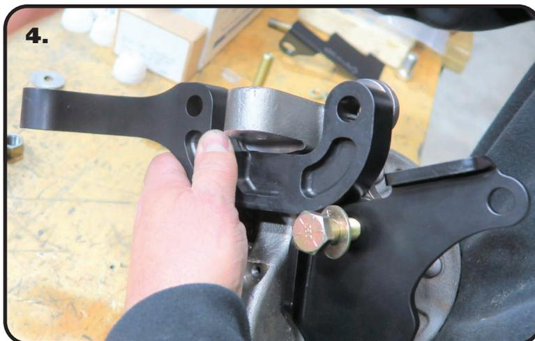
4. Align the Steering Arm mounting holes with the 2 bottom holes of the spindle. The steering arm will be pointing the opposite direction of the caliper bracket. Again, this is the passenger side with the steering arm going to the rear of the car.
