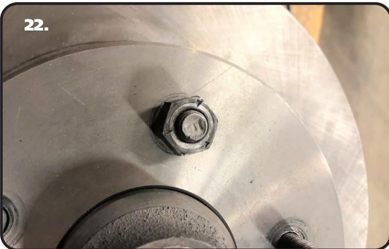
**22.** To help ease caliper installation, thread a lug nut onto a stud to hold the rotor in place.
