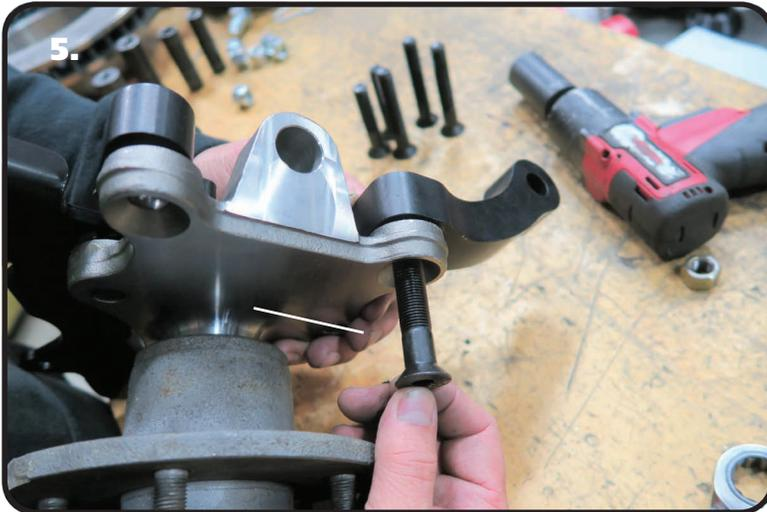
5. Insert (1) 1/2"-13 x 2 1/2" flat head socket cap screws through the spindle and steering arm. Install a 1/2"-20 nylok nut on the bolt closest to the end that attaches the tie rod.
