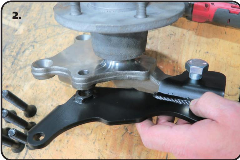
2. Apply Red Loctite to the 5/8" -18 x 1" bolt supplied with the spindle. Using **Image 2** as a reference, line up the 5/8" hole of the bracket with the threaded hole near the top of the spindle. Insert the 5/8" bolt through the hole in the bracket and thread it into the spindle. Pictured is the passenger assembly, it positions the caliper on the front side of the spindle
