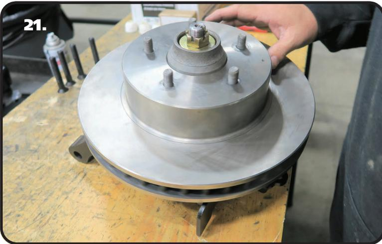
**21.** Install the OEM rotor onto the hub.
