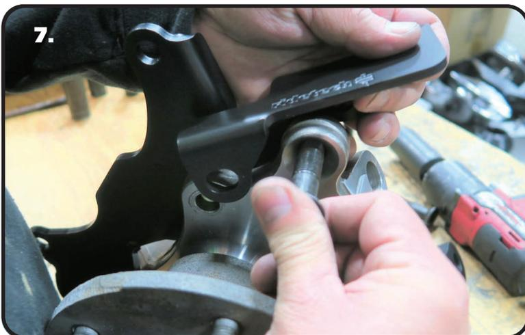
7. Align the steering arm and steering stop with the hole in the spindle.
