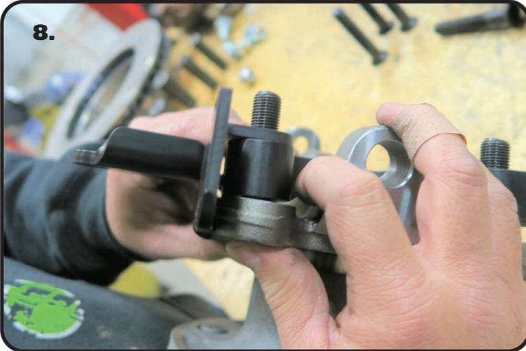
**8.** Insert a 2nd 1/2"-20 x 2 1/2" flat head socket cap screw through the spindle, steering arm, and steering stop. Install a 1/2"-20 nylok nut.
