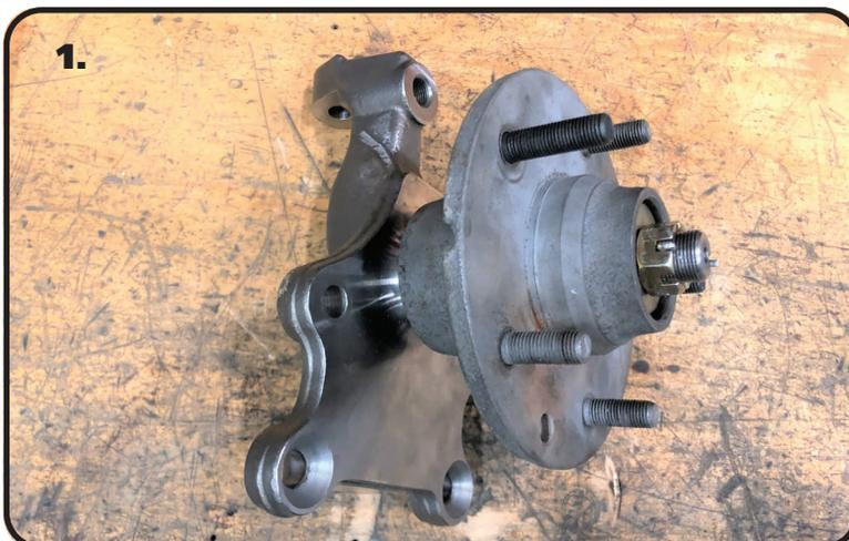
**1.** Start by greasing the wheel bearings and installing the hubs on the spindle using the nut, washer, and cotter pin supplied with the kit.
