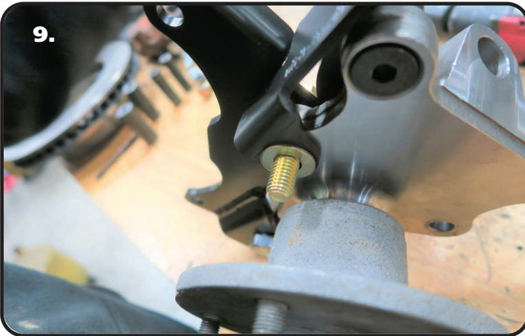
**9.** Push the 1/2"-20 x 2 1/4" bolt through the tab of the steering stop. Install a 1/2" flat washer, & 1/2"-20 nylok nut. Torque the 1/2" hardware to 90 ftlbs.
