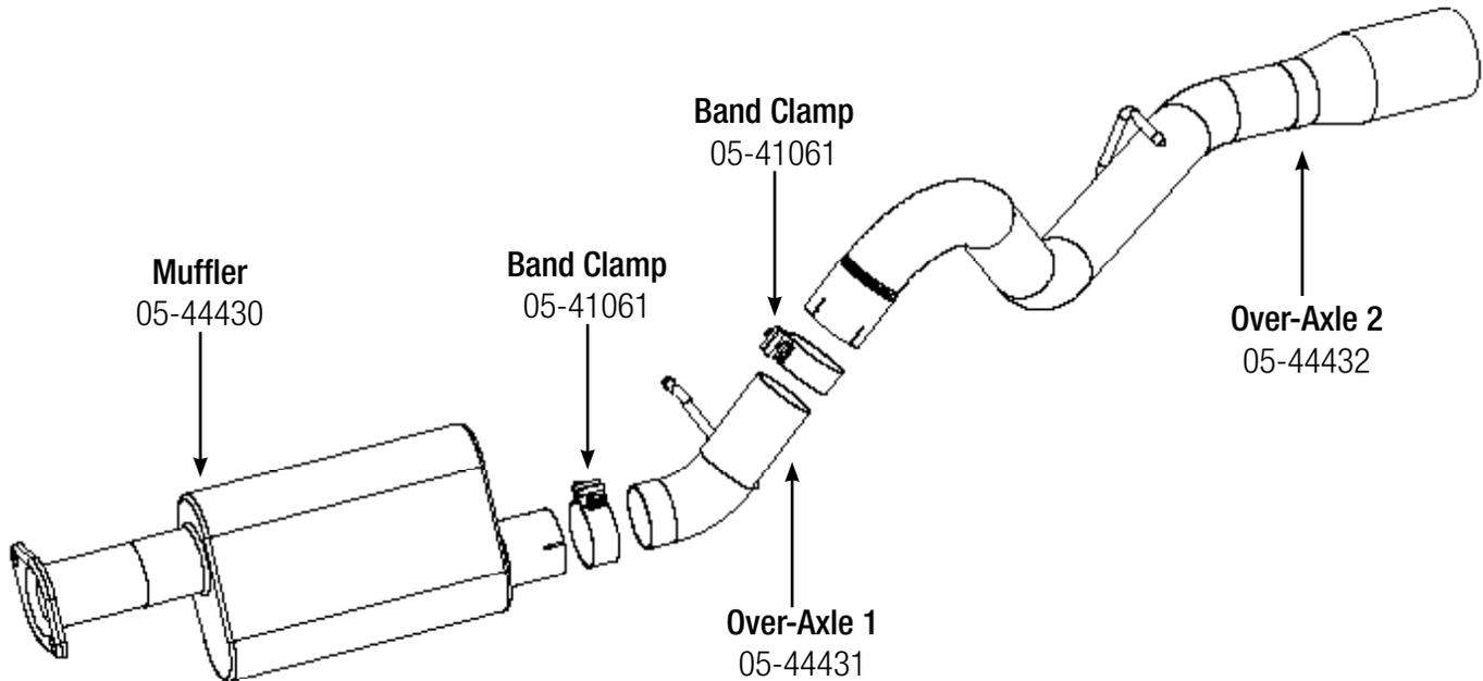
**Step 1: (Read Instructions prior to installation)** Remove your stock exhaust from the rear of your truck working your way forward. Take caution not to damage the factory isolation mounts as they will be reused. It may be helpful to lubricate the isolation mounts prior to disassembly. **It is recommended to not fully tighten the clamps until the entire system has been installed.**
