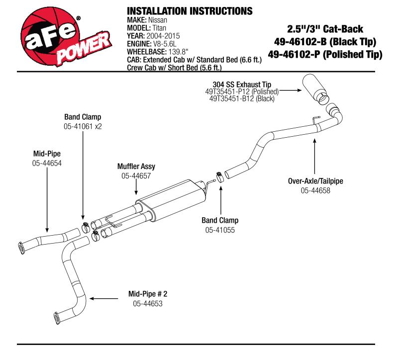
**Step 1:** (Read Instructions prior to installation) Remove your stock exhaust up to the catalytic converter from the rear of your truck working your way forward. Take caution not to damage the factory hardware and isolation mounts as they will be reused. It is recommended to not fully tighten the clamps until the entire system has been installed.
