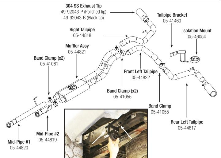
**Step 1: (Read Instructions prior to installation)** Remove your stock exhaust up to the catalytic converter from the rear of your truck working your way forward. Take caution not to damage the factory hardware and isolation mounts as they will be reused. **It is recommended to not fully tighten the clamps until the entire system has been installed.**
