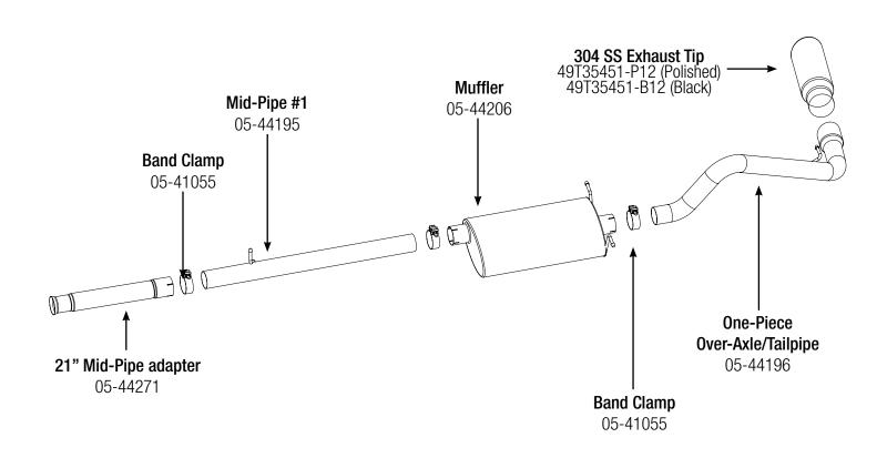
**Step 1: (Read Instructions prior to installation)** Remove your stock exhaust up to the catalytic converter from the rear of your truck working your way forward. Take caution not to damage the factory hardware and isolation mounts as they will be reused.
