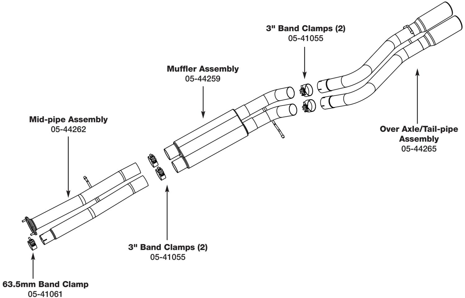
**Step 1: (Read Instructions prior to installation)** Remove your stock exhaust from the rear of your truck working your way forward, it will be necessary to cut the stock exhaust at a convenient location due to its length. Take caution not to damage the factory isolation mounts as they will be reused. **It is recommended to not fully tighten the clamps until the entire system has been installed.**
