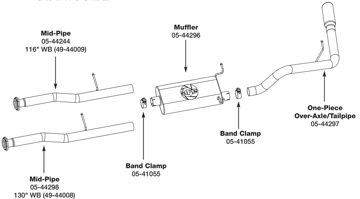
**Step 1: (Read Instructions prior to installation)** Remove your stock exhaust up to the catalytic converter from the rear of your truck working your way forward. Take caution not to damage the factory isolation mounts as they will be reused. This system is best installed with a chassis lift with axles extended for clearance. **It is recommended to not fully tighten the clamps until the entire system has been installed.**
