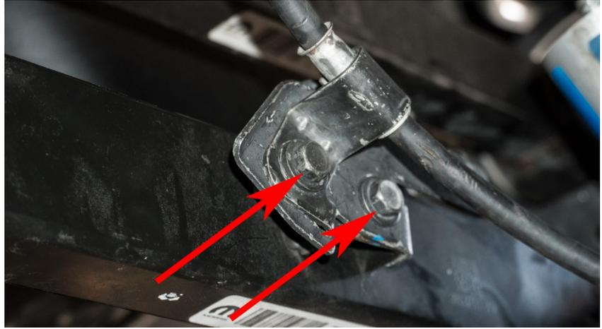
3. Remove the bracket from the passenger side cable as this will not be reused. To clarify, the bracket that connected the passenger's side brake cable to the driver's side lower control arm.
