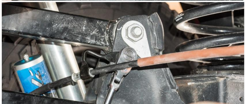
6. Install Carli Bracket to the driver's side lower control arm using the factory bolt.
