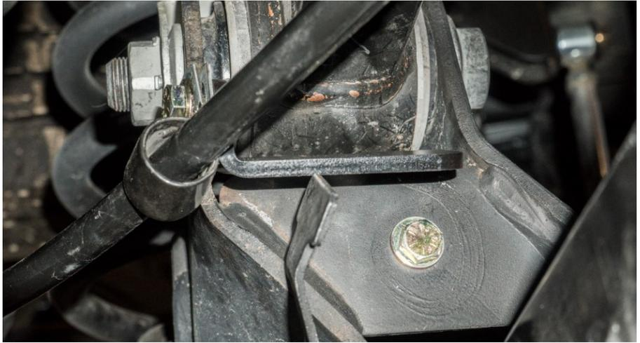
10. Use the factory bolt and the provided M10 x 30mm bolt to secure the 3-prong bracket to the top of the differential. The bracket will offset downward with the capture nut threads facing up.
