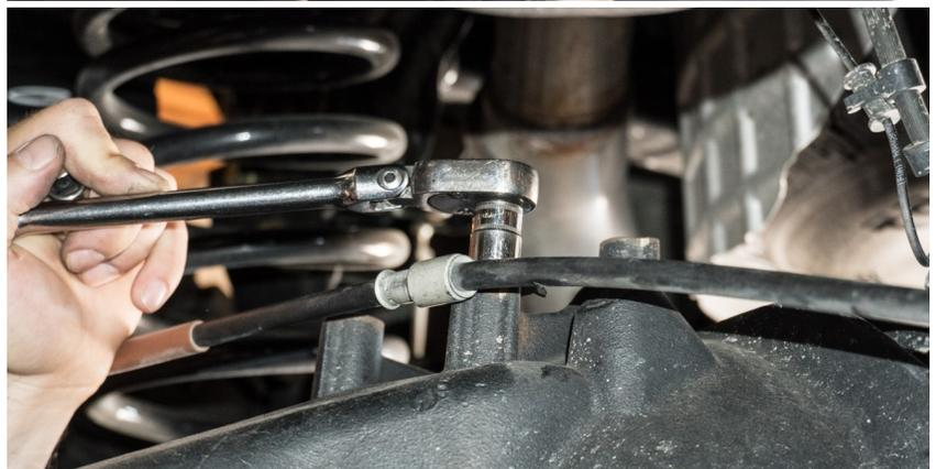
5. 13mm Socket - Remove the bolt securing the brake line bracket to the inside of the passenger's side control arm bracket.
