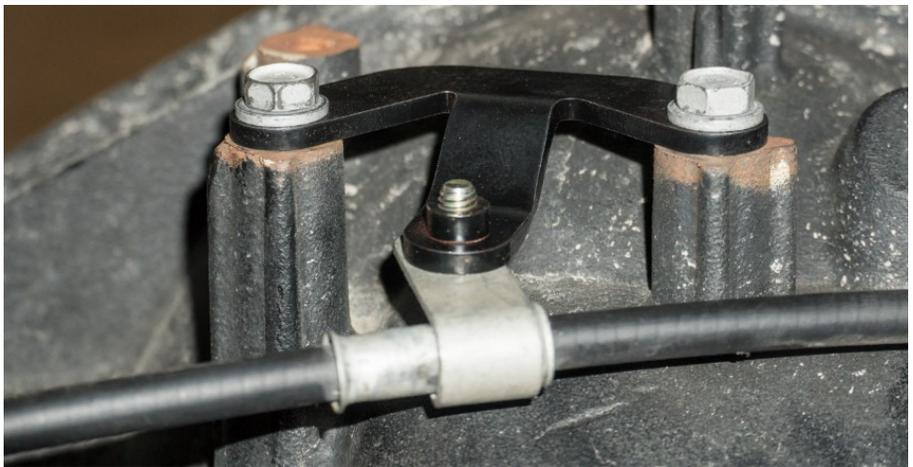
12. Use the Factory Bolt to secure the Carli Bracket to the Passenger-Side Inner Control Arm mount.
