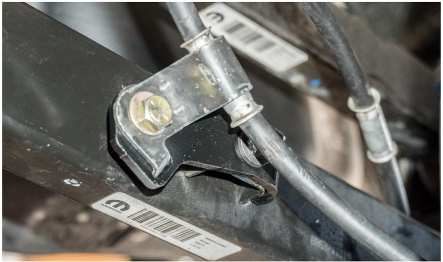
8. Install the Carli Bracket to the rear, upper control arm mount. Slide the capture-nut end of the Carli bracket into the control arm bracket and secure in place using the provided 5/16" x 3/4" bolt and washer through the existing hole between the control arms.
