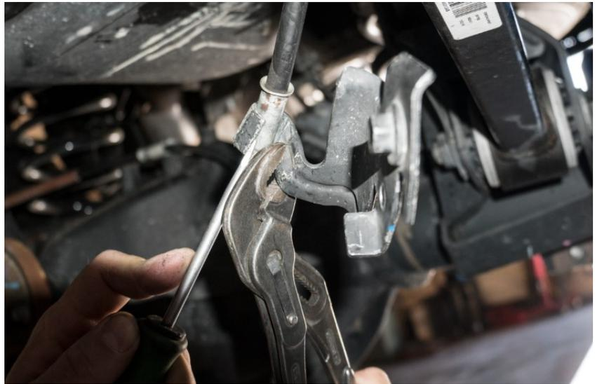
4. 15mm Socket - Remove the bolt securing the factory brake line tab to the top of the differential.
