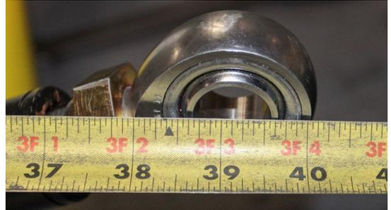
16. Confirm ends remained parallel during torquing and note the position of the jam nut. The flat part of the "hex" on the jam nut is indexed so it is parallel to the rod-end's orientation. This will ensure that the jam nut does not rub the factory track bar pocket. If the "point" of the jam nut faces the rear of the track bar, the jam nut will rub the bracket and could loosen.
