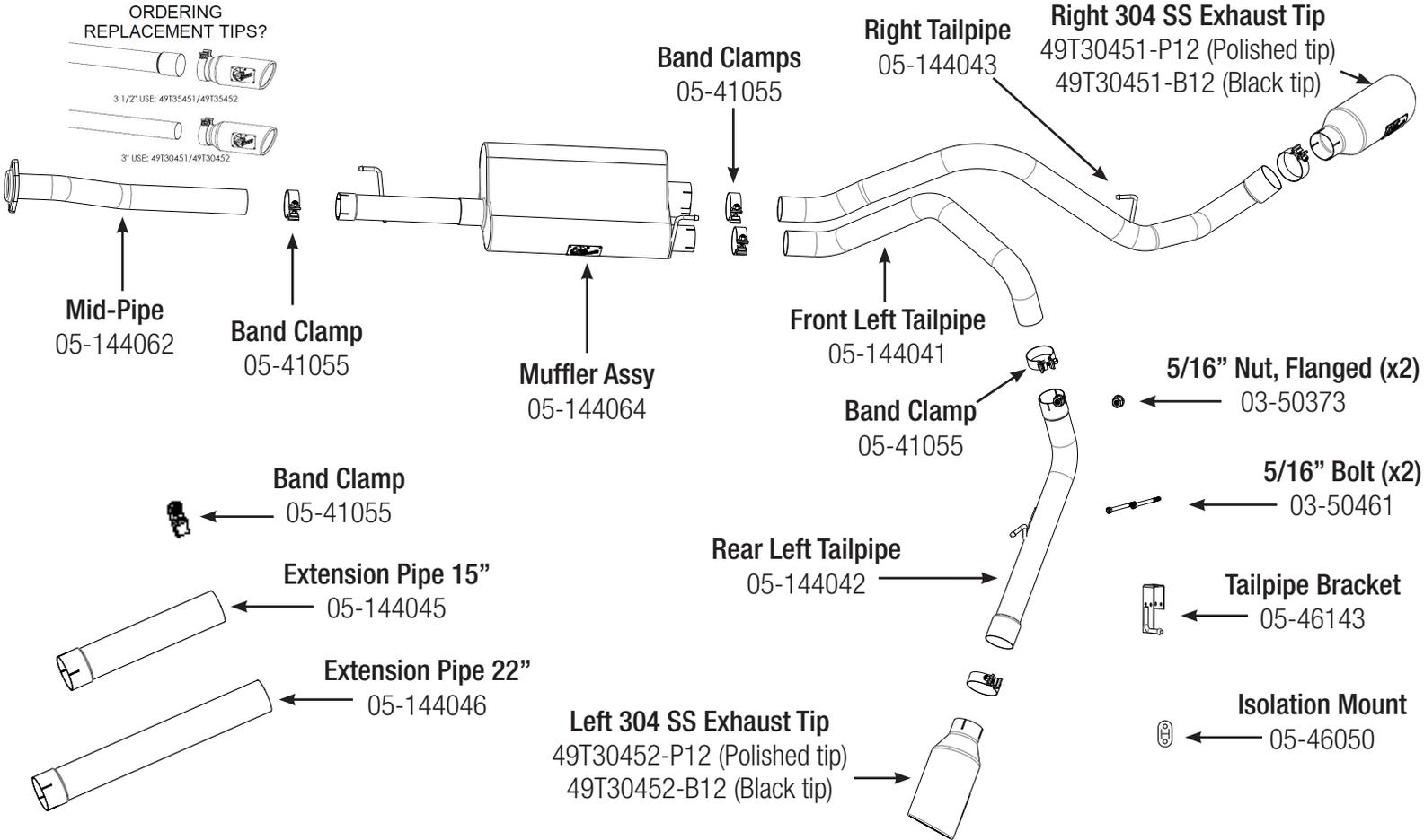
**Step 8:** Install the Hanger Bracket included with the kit. As shown on **(figure A)**. Fully tighten the hanger bracket to the frame using the correct hardware provided.
