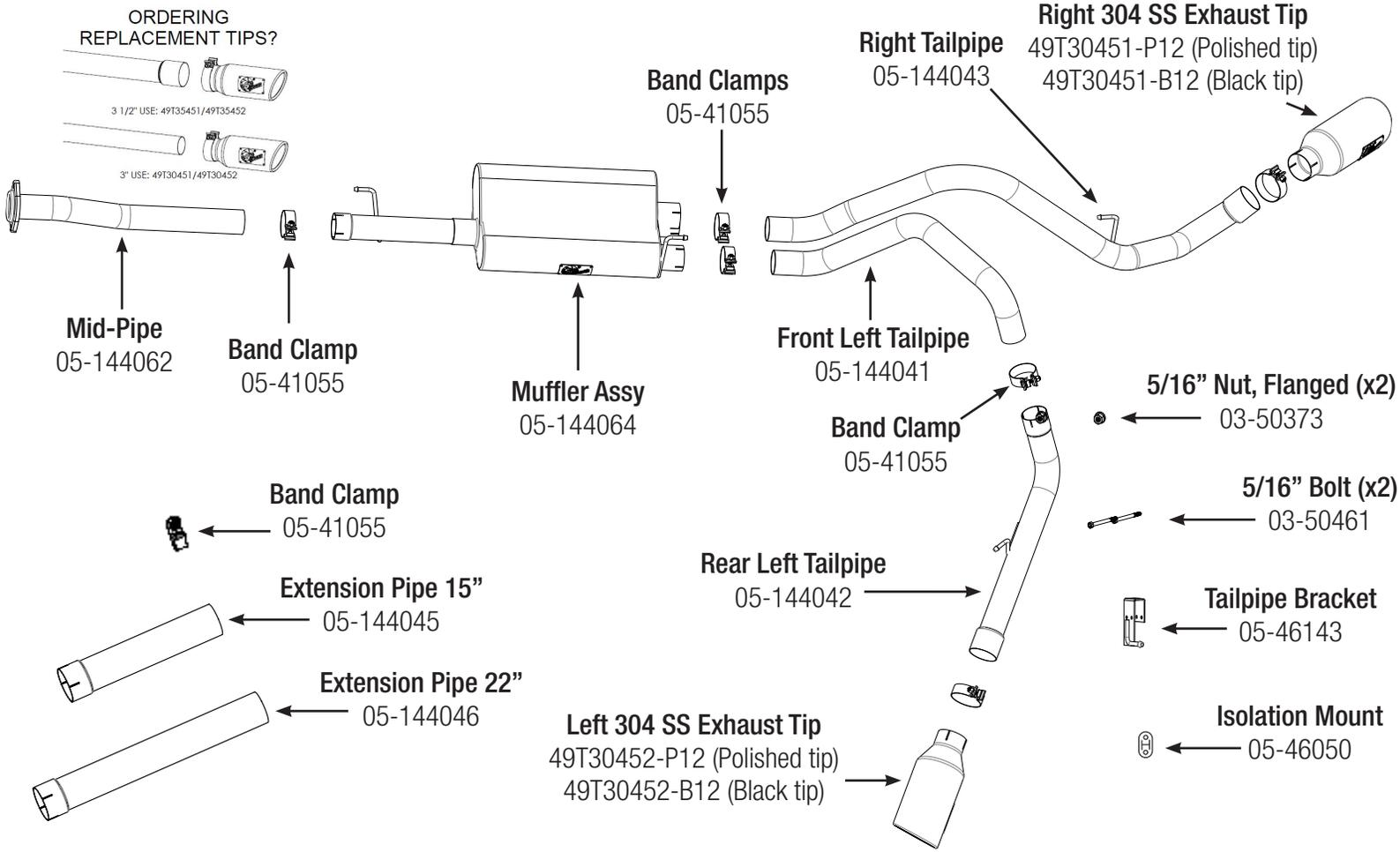
**Step 1:** (Read Instructions prior to installation) remove your stock exhaust up to the catalytic converter from the rear of your truck working your way forward. Take caution not to damage the factory hardware and isolation mounts as they will be reused. It is recommended to not fully tighten the clamps until the entire system has been installed.
