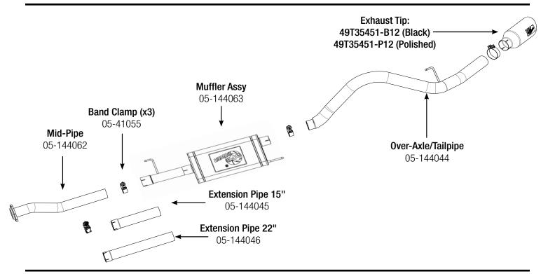
**Step 1:** (Read Instructions prior to installation) Remove your stock exhaust up to the catalytic converter from the rear of your truck, working your way forward. Take caution not to damage the factory hardware and isolation mounts as they will be reused. (it is recommended to not fully tighten the clamps until the entire system has been installed.)
