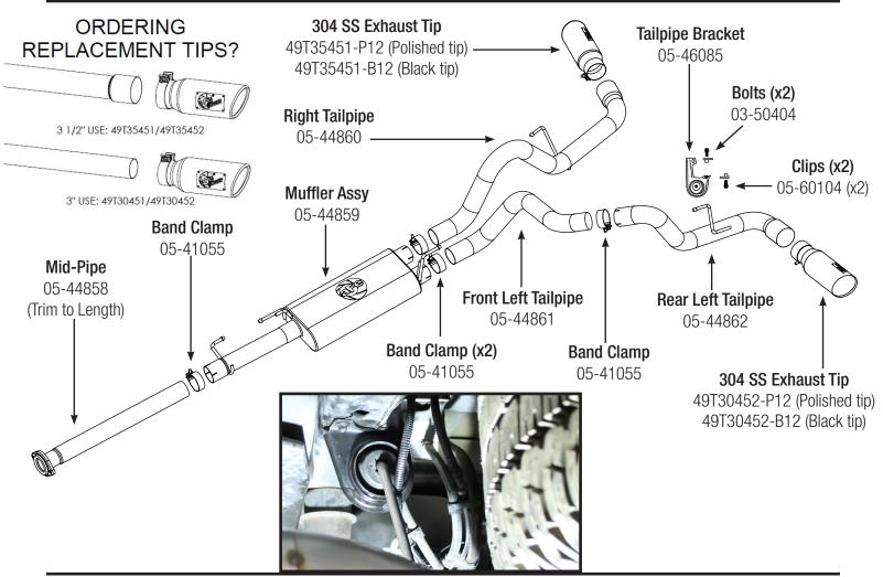
**Step 1: (Read Instructions prior to installation)** Remove your stock exhaust up to the catalytic converter from the rear of your truck working your way forward. Take caution not to damage the factory hardware and isolation mounts as they will be reused.
