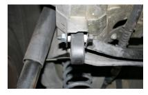
**Step 6:** Install the supplied hanger rod assembly, (x1) rubber hanger mount and 8 x 1.25 bolt to the chassis and tighten.
