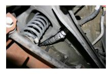
**Step 8:** Install the aFe Front Mid Pipe using the original band clamp from step 4 but do not tighten.
