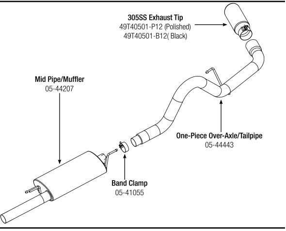
**Step 1: (Read Instructions prior to installation)** Remove your stock exhaust up to the catalytic converter from the rear of your truck working your way forward. Take caution not to damage the factory hardware and isolation mounts as they will be reused.
