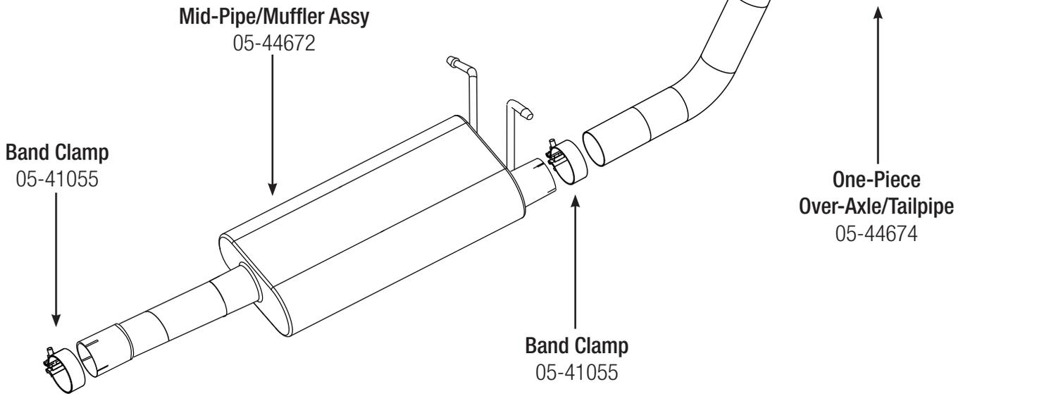
**Step 1: (Read Instructions prior to installation)** Remove your stock exhaust from the rear of your truck working your way forward. It may be necessary to cut the pipes if the slip joints are stuck. Do not cut the pipe after the cat. You will be using this slip connection. Take caution not to damage the factory isolation mounts, as they will be reused. It is recommended to not fully tighten the clamps until the entire system is installed.
